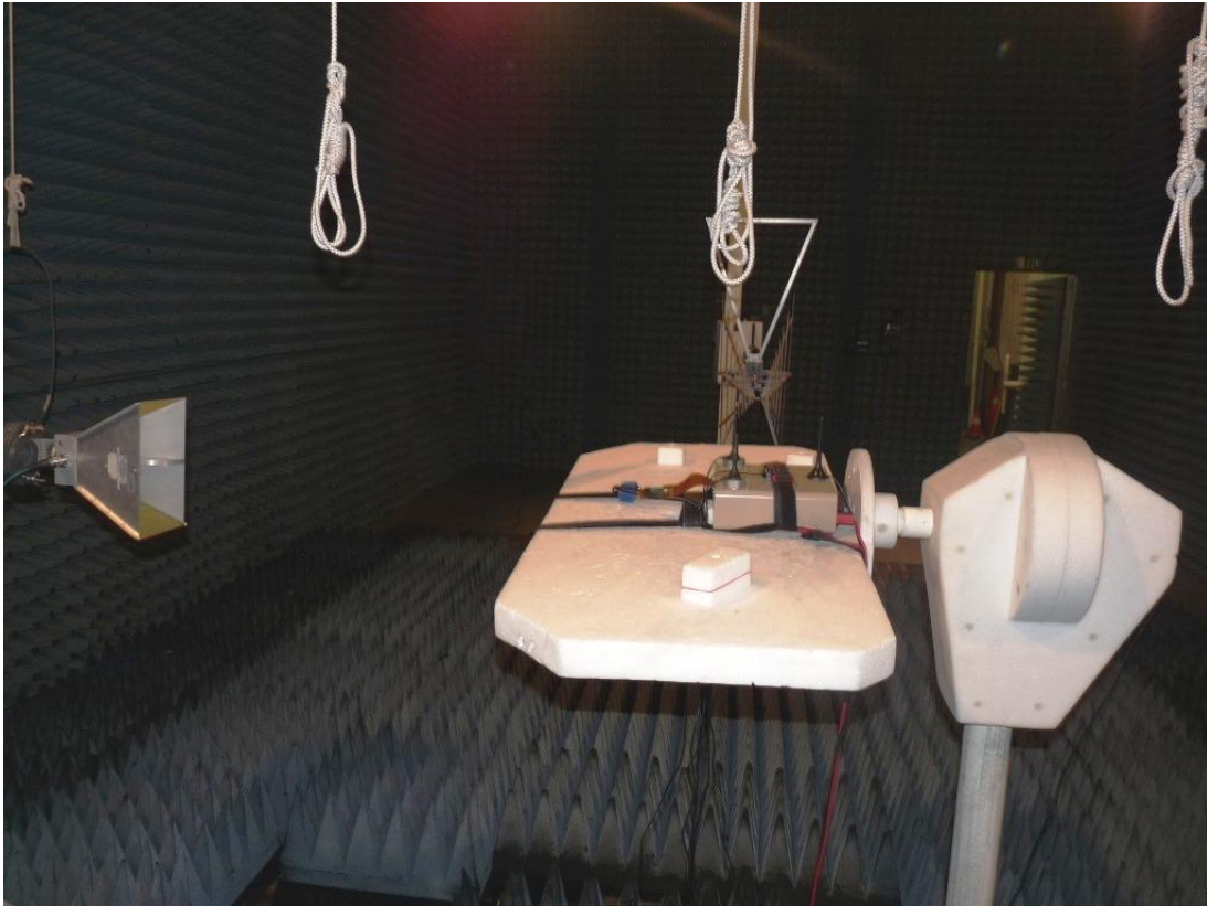
Photo 1: Test setup for radiated measurements (Enclosure, fully-anechoic chamber, 30 MHz – 10/20 GHz §90)
