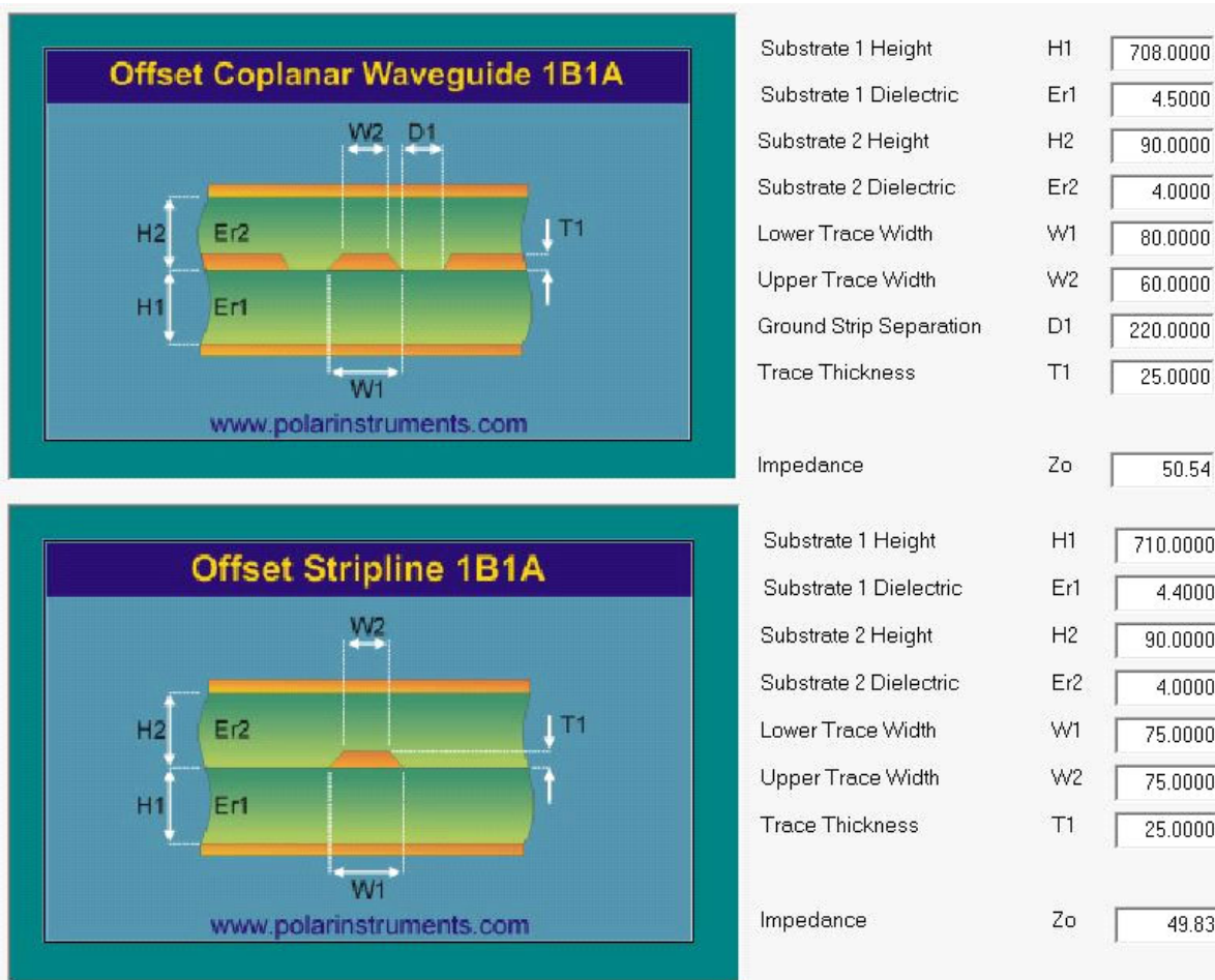
Figure 16: Embedded stripline arrangement example
