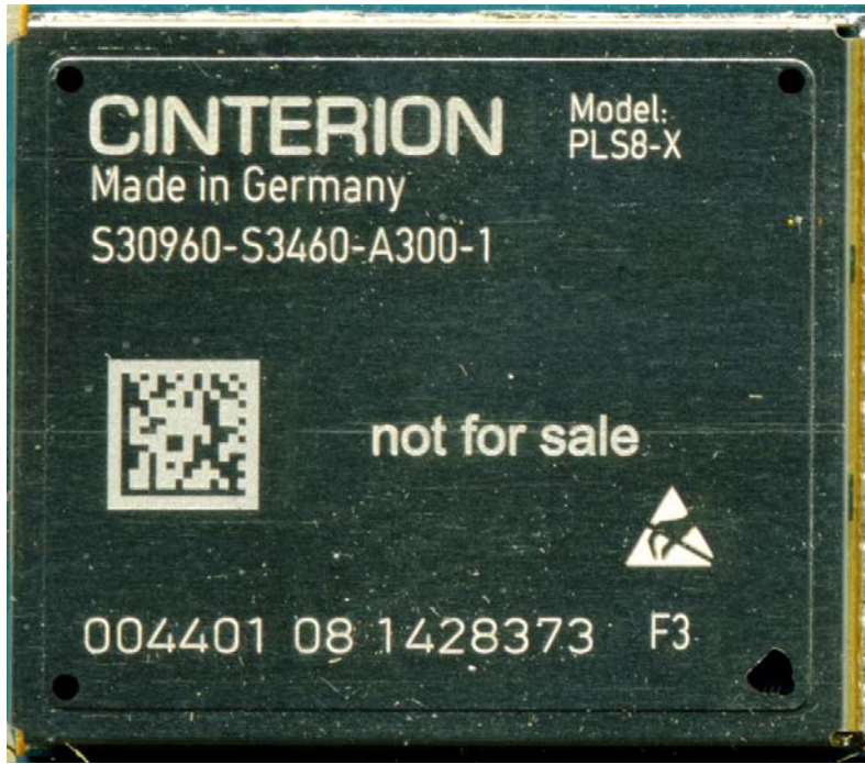
PLS8-X label location lasing on shielding
