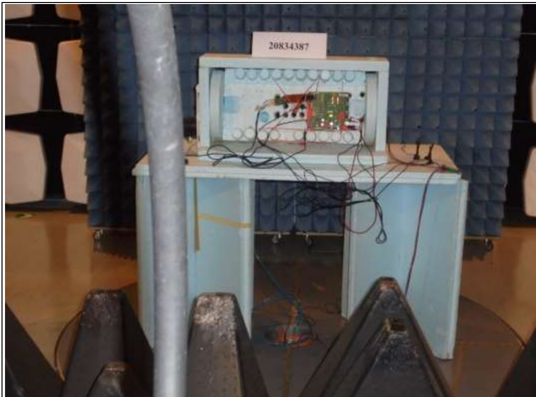
Photograph 2: Magnetic field measurements
