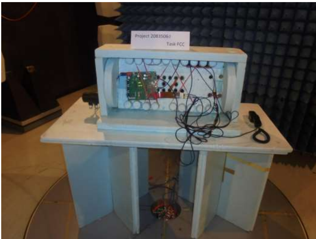
Photograph 4: Radiated mission measurements (overview)
