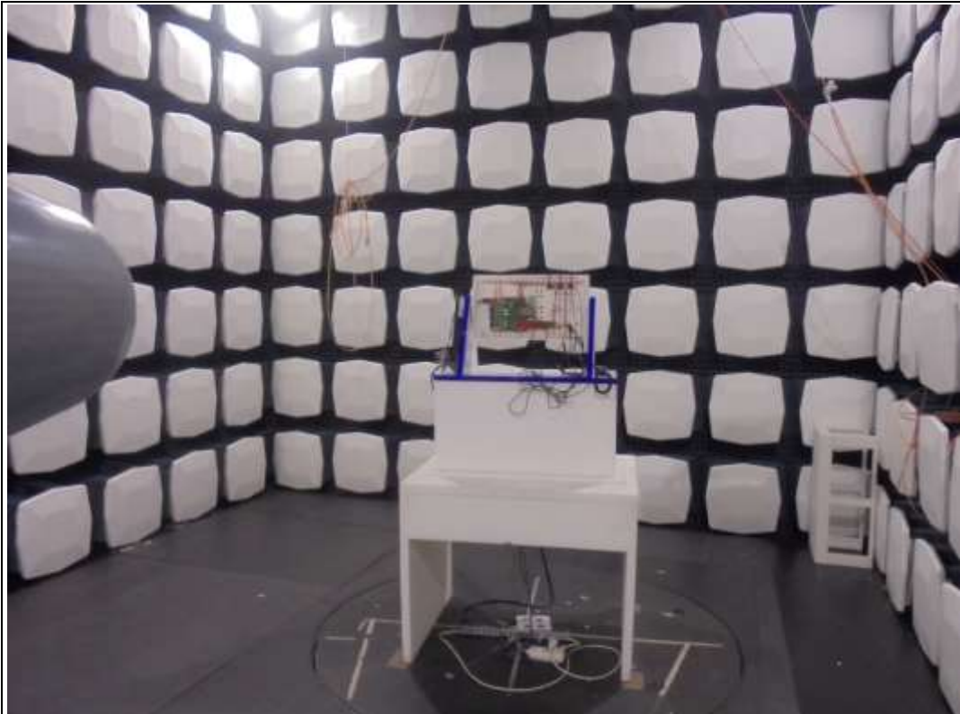
Photograph 5: Radiated mission measurements (overview)
