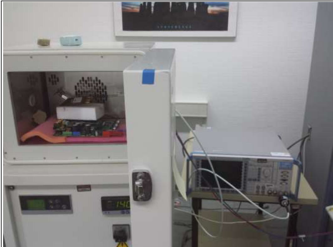
Photograph 1: Conducted measurements - Frequency error
