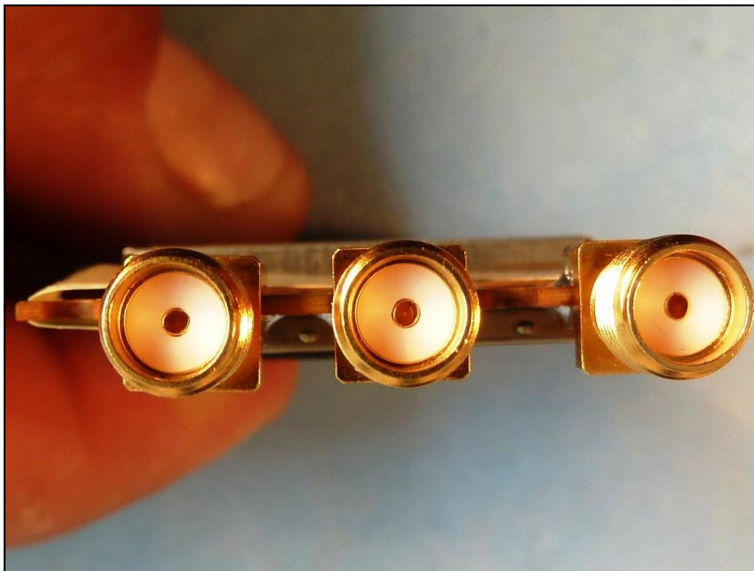
Photo 3: connectors of the EUT
