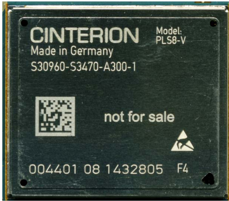
PLS8-V label location lasing on shielding
