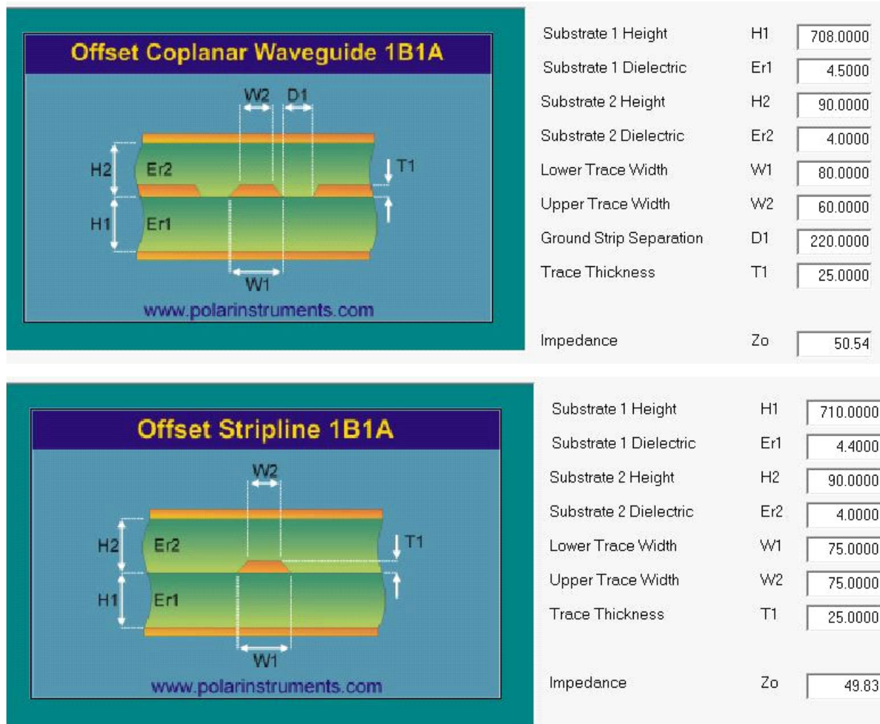
Figure 19: Embedded stripline arrangement example
