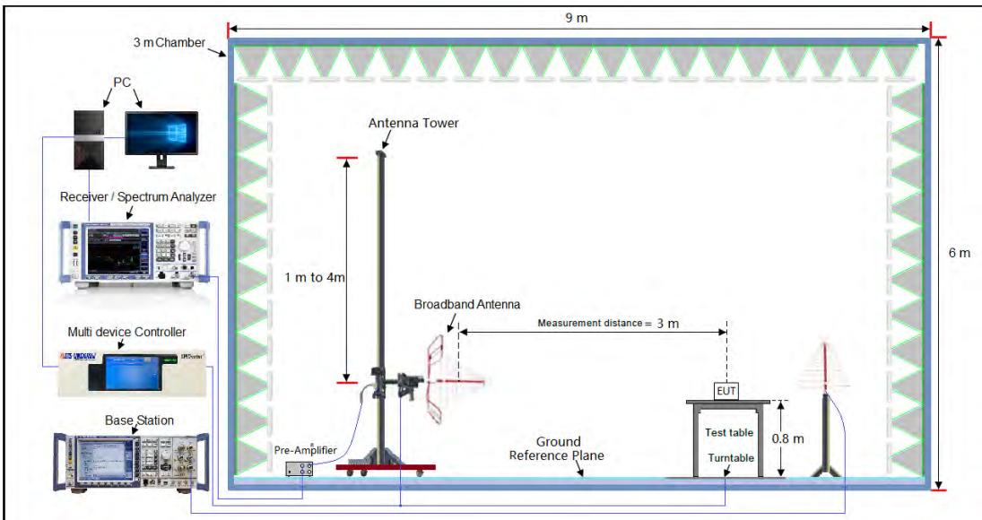
**Radiated Emissions Above 1GHz Test setup**
