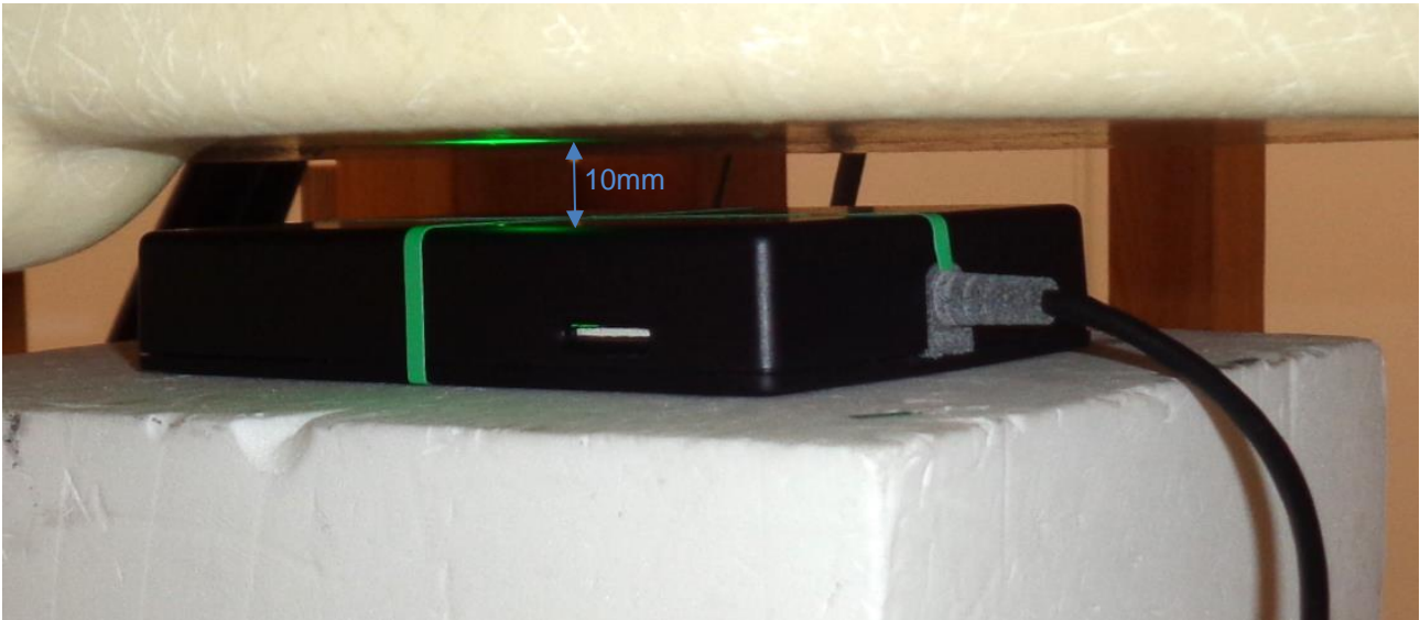
Front side of the device against the phantom with 10mm separation.
