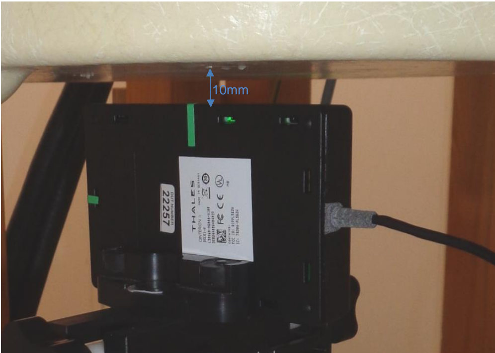
Left side of the device against the phantom with 10mm separation.
