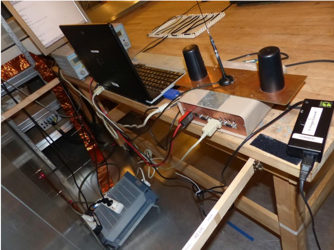
Photo 2: Test setup for radiated measurements, unintentional radiator §15) single device setup, computer peripheral.
