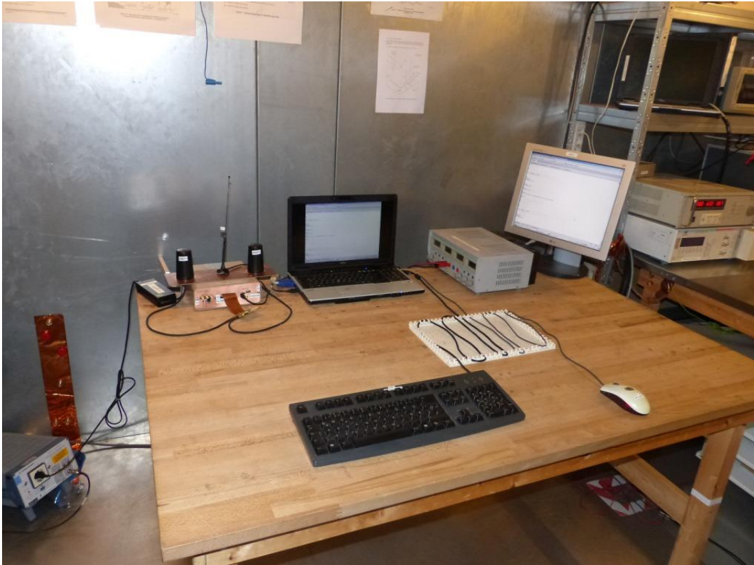
Photo 1: Test setup for radiated measurements unintentional radiator §15) Single device setup, computer peripheral.
