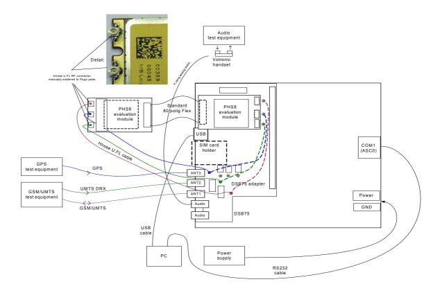
Figure 11: Reference equipment for type approval
