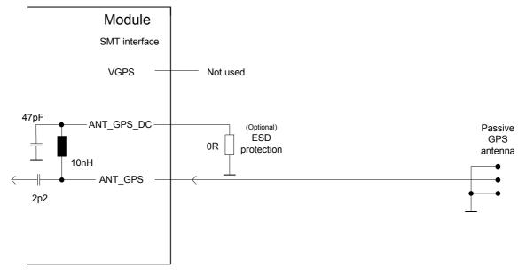
Figure 7: ESD protection for passive GPS antenna
