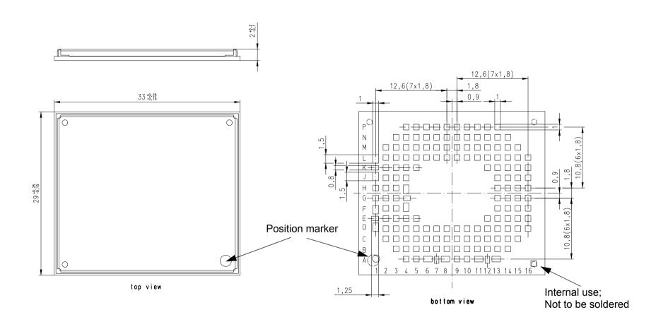
Figure 9: Dimensions of PHS8-US (all dimensions in mm)
