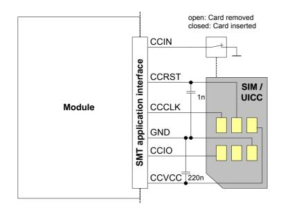
Figure 5: UICC/SIM/USIM interface
