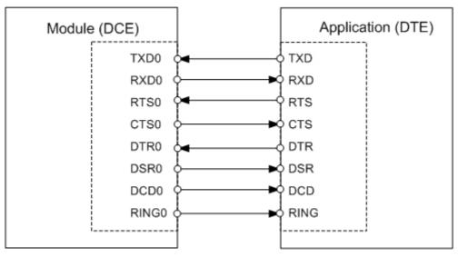
Figure 4: Serial interface ASC0
