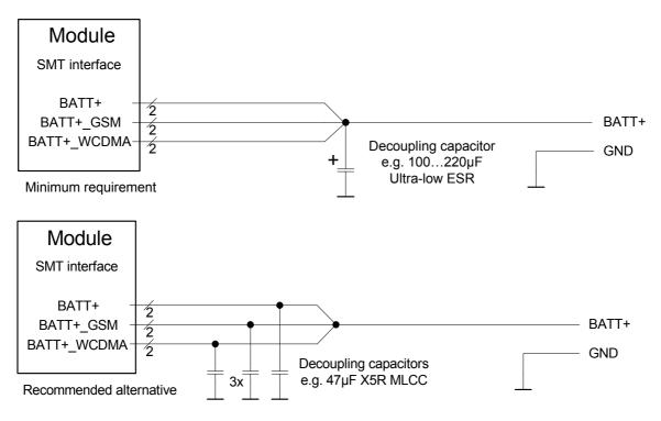
Figure 2: Decoupling capacitor(s) for BATT+
