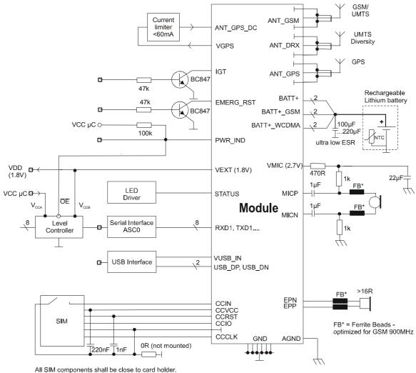
Keep SIM wires low capacitive.
