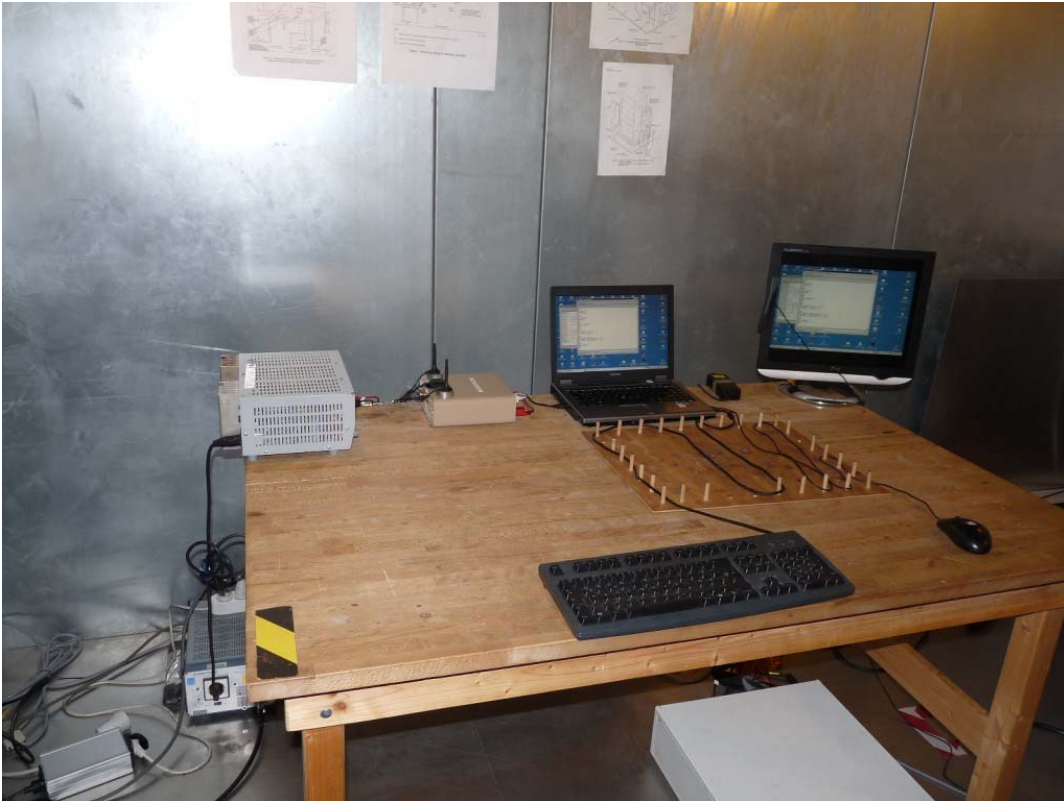
Photo 4: Test setup for conducted measurements (AC Port (power line)), computer peripheral setup
