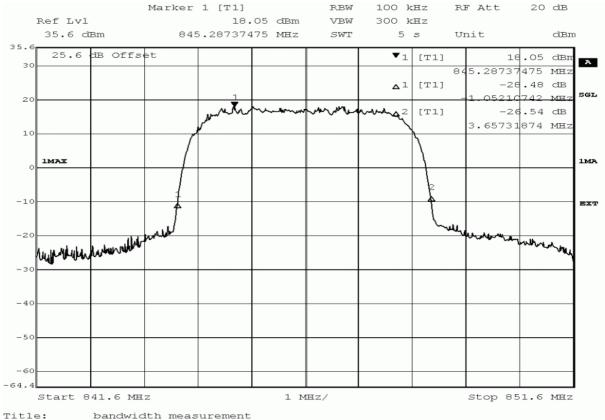
bandwidth measurement Comment A: CZ400, FDD V, 26dB bandwidth, channel 4233 (846.6MHz)
