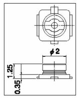
Figure 5: Mechanical dimensions of PH8/PH8-P antenna connectors
