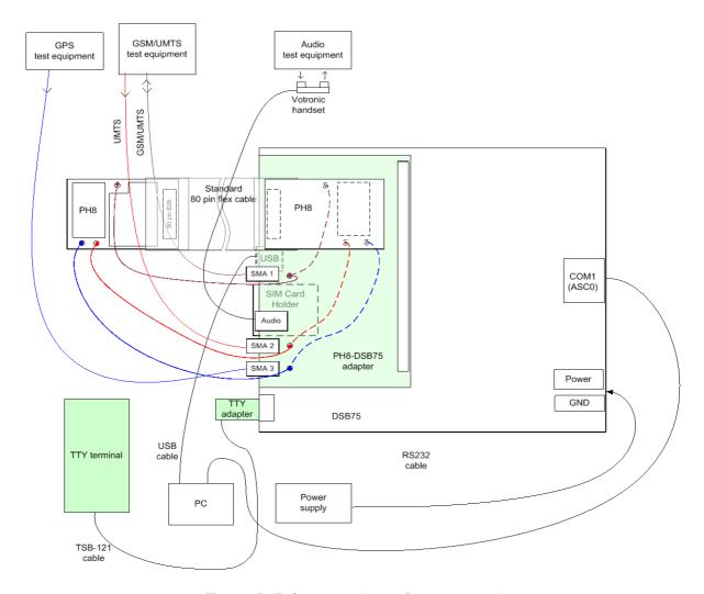
Figure 15: Reference equipment for type approval
