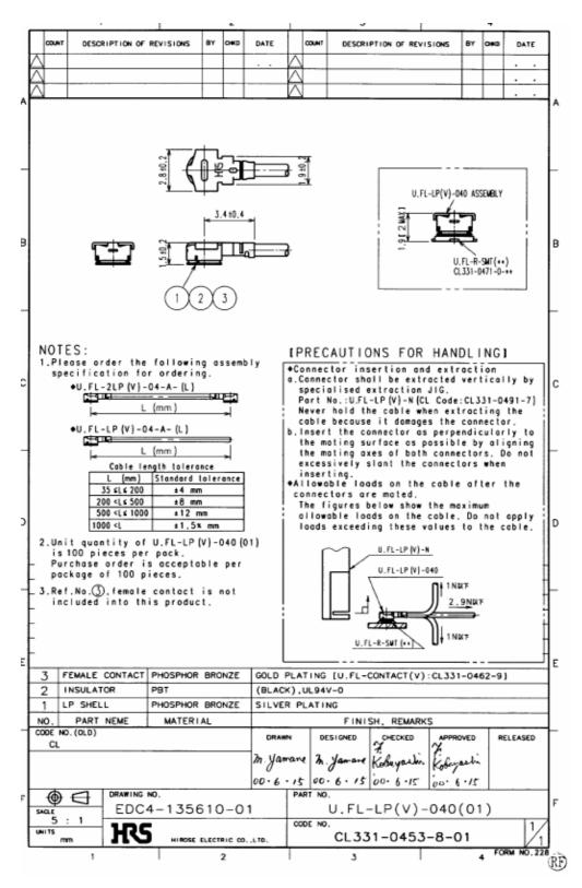
Figure 8: Specifications of U.FL-LP-(V)-040(01) plug
