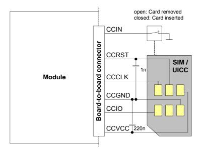
Figure 4: UICC/SIM/USIM interface
