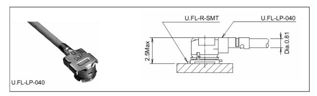
Figure 6: U.FL-R-SMT connector with U.FL-LP-040 plug
