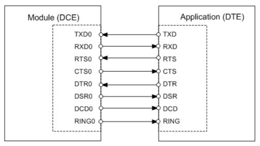
Figure 3: Serial interface ASC0
