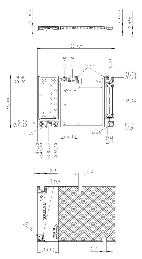
Figure 10: Dimensions of PH8/PH8-P (all dimensions in mm)
