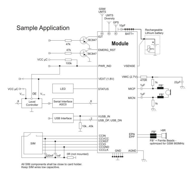
Figure 14: PH8/PH8-P sample application
