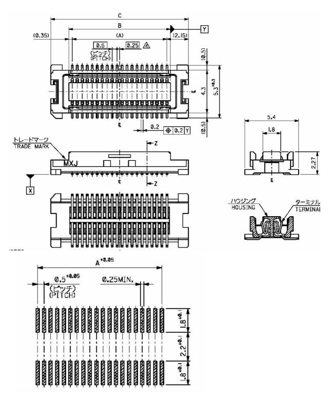
Figure 12: Molex board-to-board connector 52991-0808 on PH8/PH8-P
