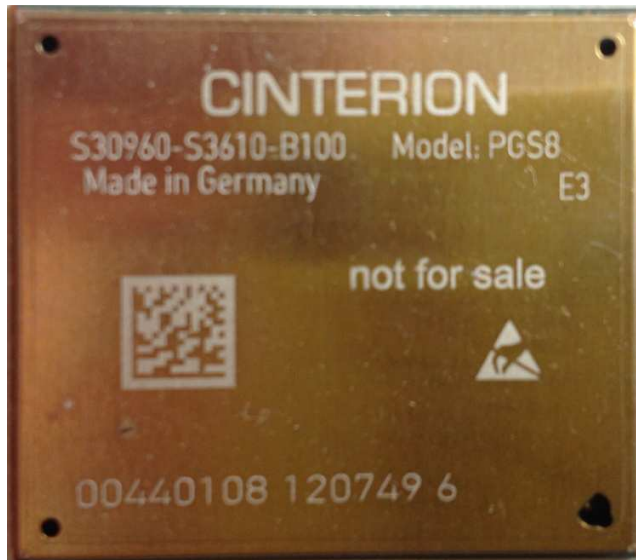
PGS8 label location lasing on shielding
