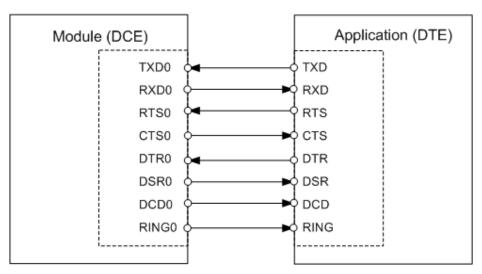
Figure 3: Serial interface ASC0
