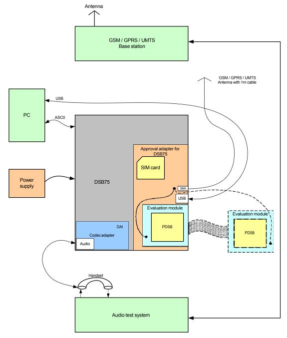
Figure 7: Reference equipment for Type Approval
