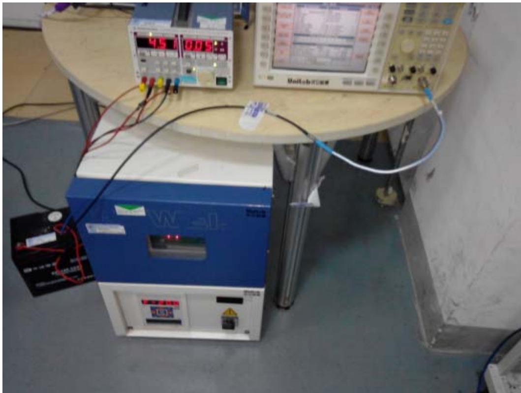
Frequency Stability Under Temperature & Voltage Variations Setup
