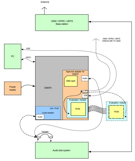
Figure 7: Reference equipment for Type Approval
