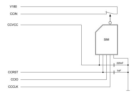
Figure 4: External UICC/SIM/USIM card holder circuit
