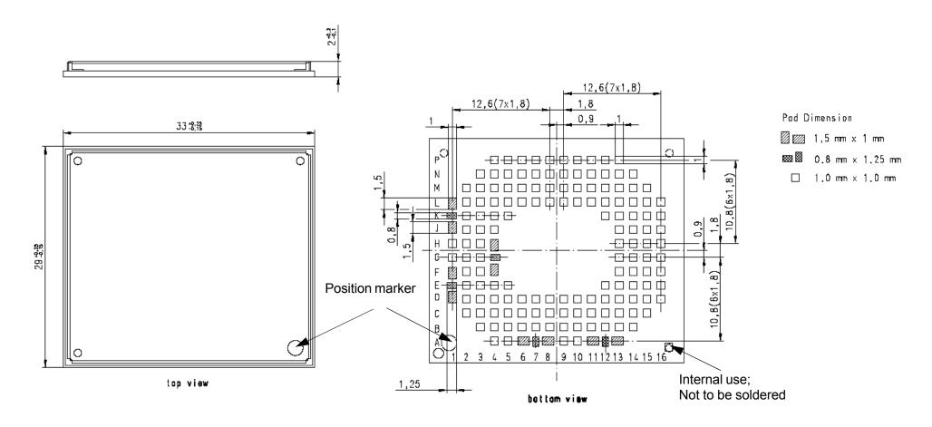
Figure 6: Dimensions of PDS6 (all dimensions in mm)
