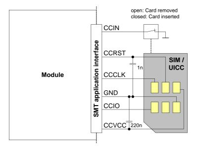
Figure 4: External UICC/SIM/USIM card holder circuit
