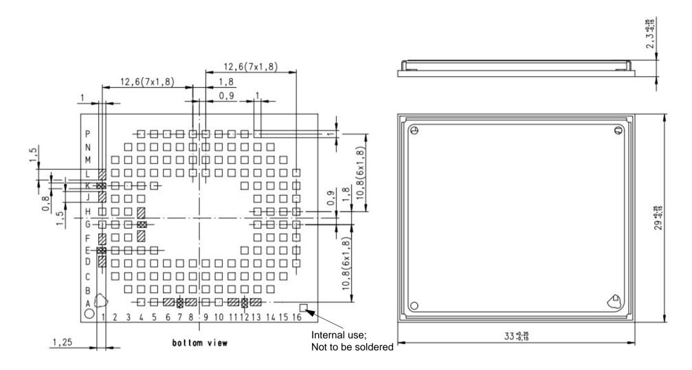
Figure 6: Dimensions of PDS5-E/PDS5-US (all dimensions in mm)
