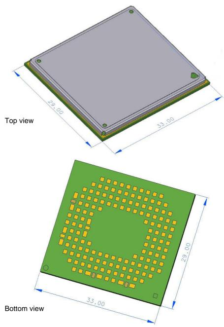
Figure 5: PDS5-E/PDS5-US - top and bottom view
