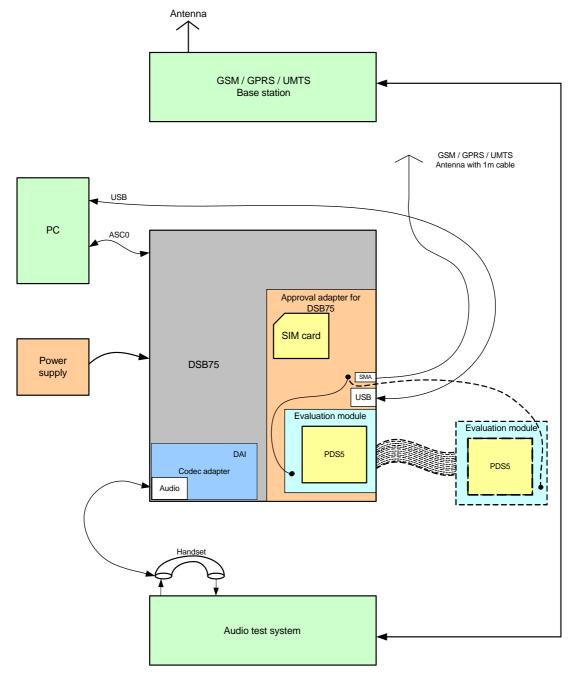
Figure 7: Reference equipment for Type Approval
