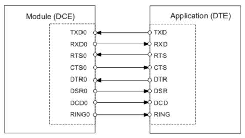
Figure 3: Serial interface ASC0
