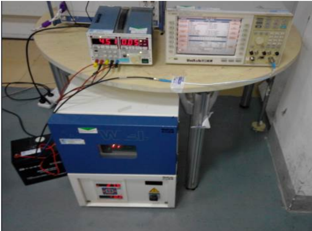
Frequency Stability Under Temperature & Voltage Variations Setup
