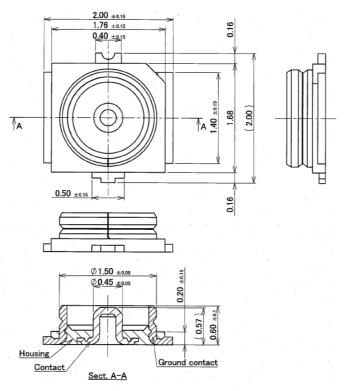
Figure 18: UMTS/LTE & Sub 6G Antenna Connector (male)
