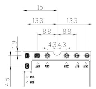
Figure 17: Antenna Interfaces
