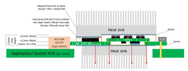
Figure 22: Option 3 - Heat sink on top of stepped shielding and directly on bottom of M.2 card PCB
