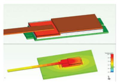
Figure 25: Thermal distribution with a heat pipe
