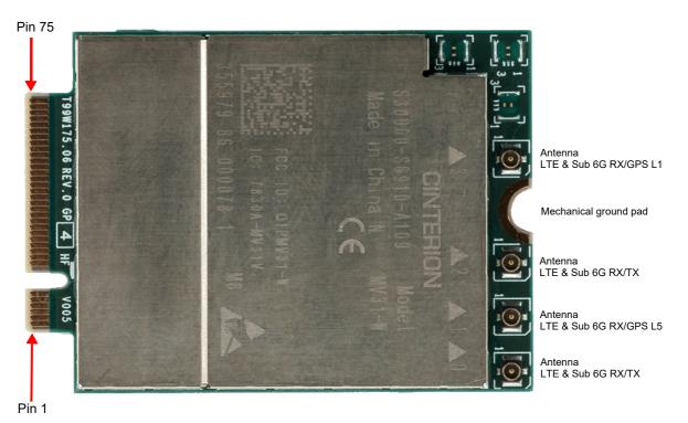
Figure 1: 5G M.2 Data Card MV31-W top view
