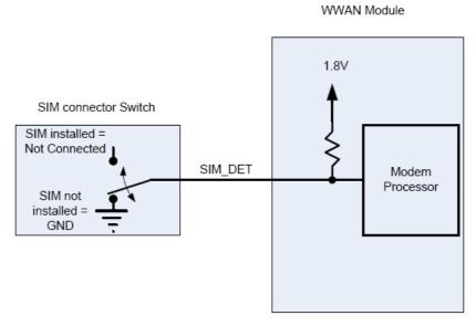
Figure 14: SIM Detection Circuit
