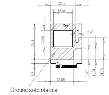
Figure 5: 5G M.2 Data Card MV31-W Ground area (with gold plating) on bottom side
