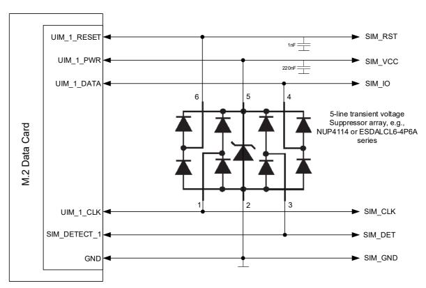
Figure 15: SIM interfaces - enhanced ESD protection
