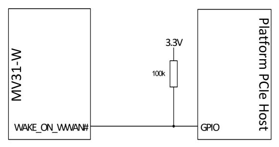
Figure 10: Typical Wake up schematic
