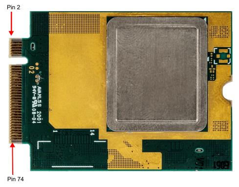
Figure 2: 5G M.2 Data Card MV31-W bottom view
