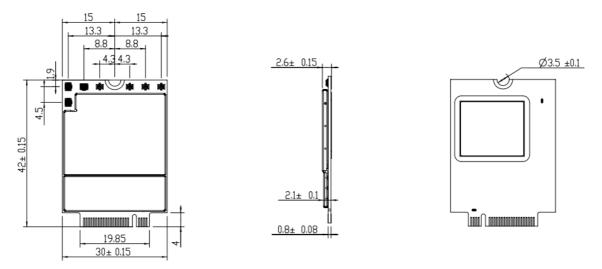
Figure 4: 5G M.2 Data Card MV31-W Dimensions
