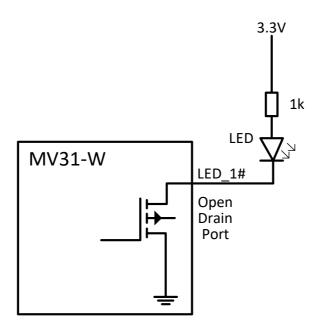
Figure 16: Sample Circuit for Status LED
