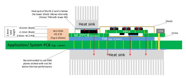
Figure 21: Option 2 - Heat sink only on heat spot of stepped shielding and bottom of application PCB
