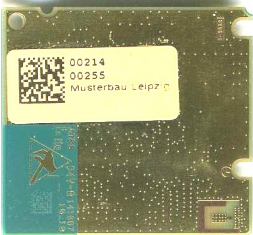
Siemens Cellular Engine MC55i Bottom Side
