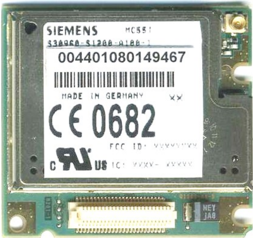
Siemens Cellular Engine MC55i Top side
