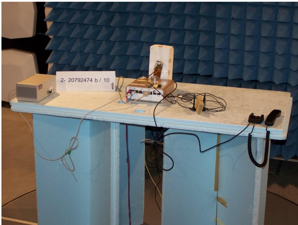
Photograph 2: Radiated measurement set-up at SAR (Semi-Anechoic-Room)
