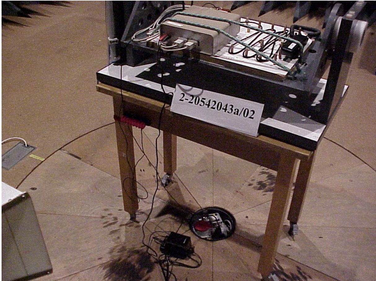
Photograph 5: Test setup for radiated emissions
