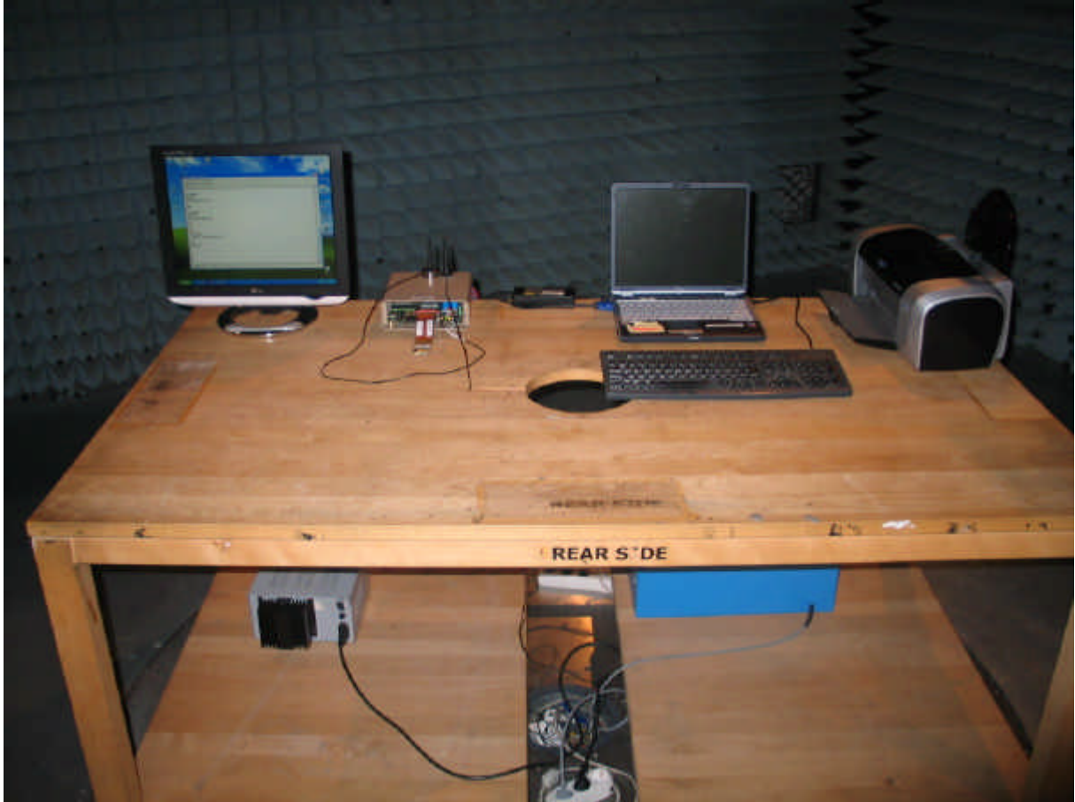
Photo 1: Test setup for radiated measurements
