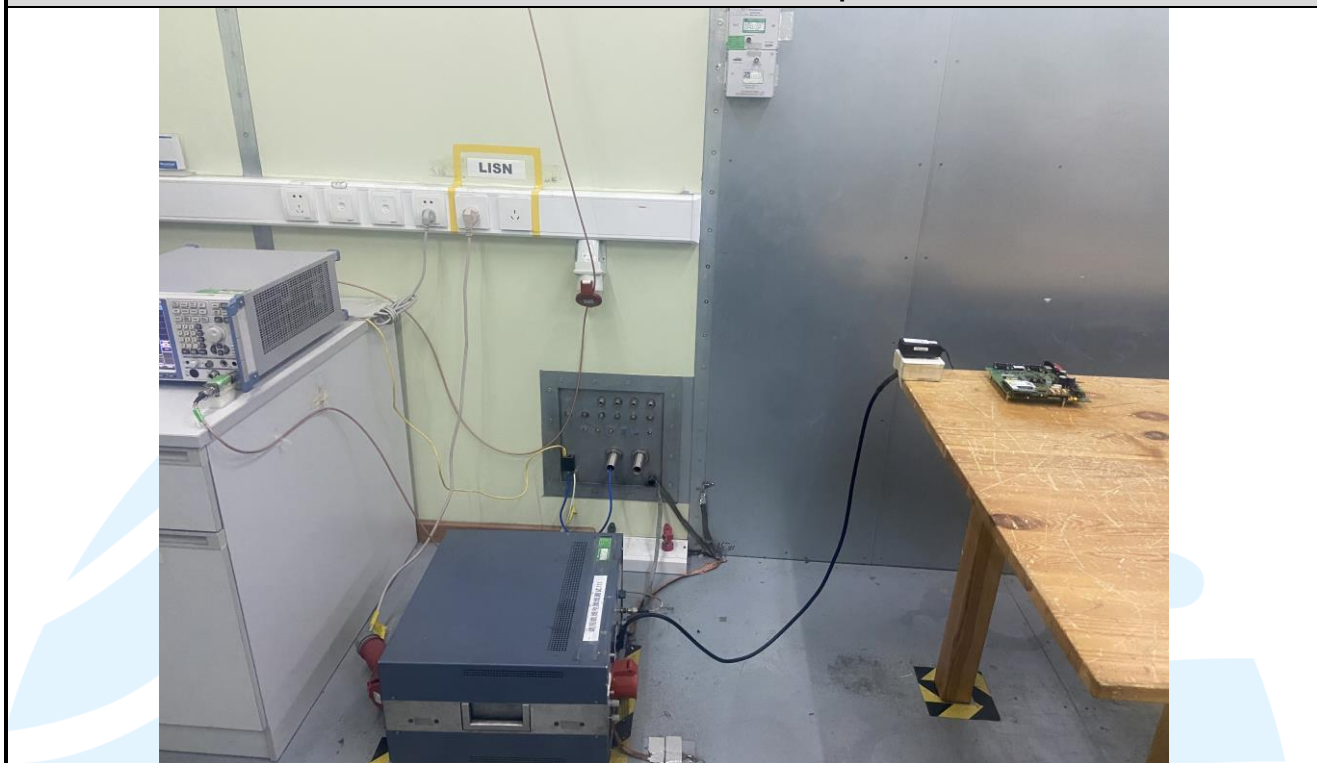
Conducted Emission Test Setup-3
