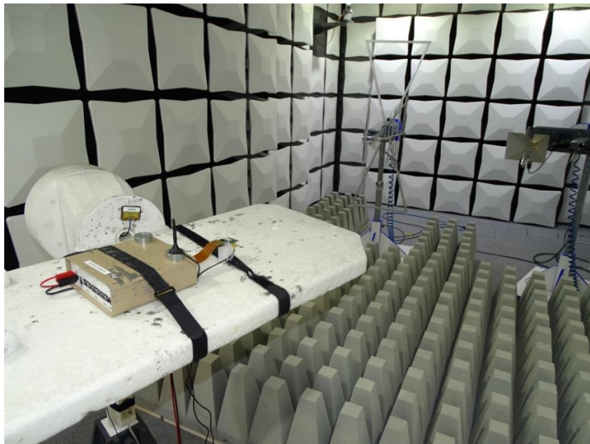
Photo 2: Test setup for radiated measurements above 1 GHz
