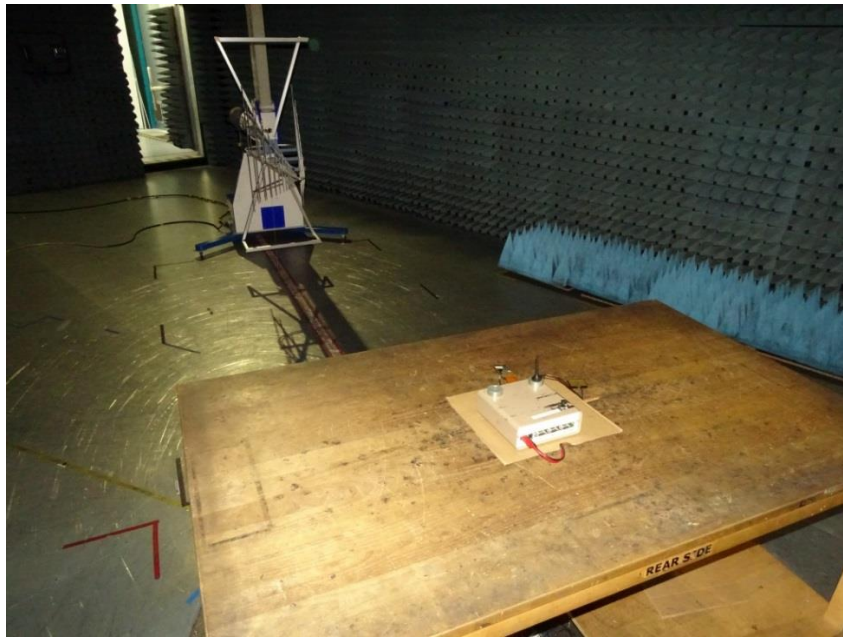
Photo 1: Test setup for radiated measurements below 1 GHz
