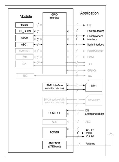
Note: The following features are not yet available with the current product release: GPIO, I<sup>2</sup>C, Pulse Counter, PWM, SPI, ADC and 2nd SIM/MIM. Second SIM/MIM interface is hardware prepared only.
