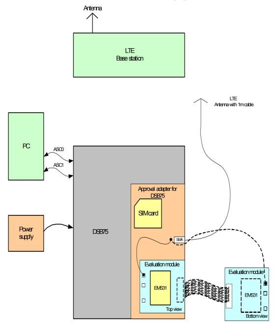
Figure 9: Reference equipment for Type Approval
