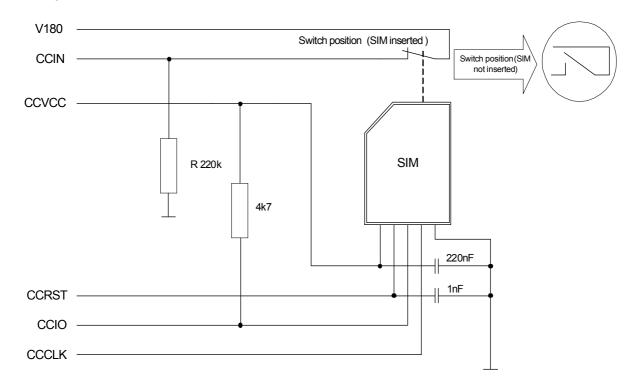
Figure 4: External UICC/SIM/USIM card holder circuit
