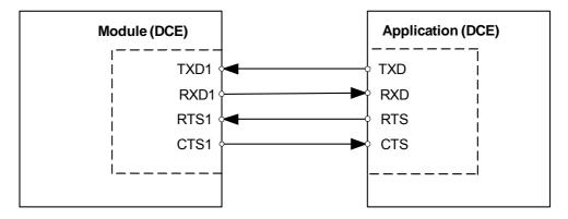
Figure 3: Serial interface ASC1
