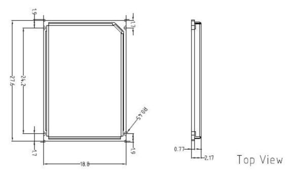
Figure 7: Dimensions of EMS31-V (all dimensions in mm)
