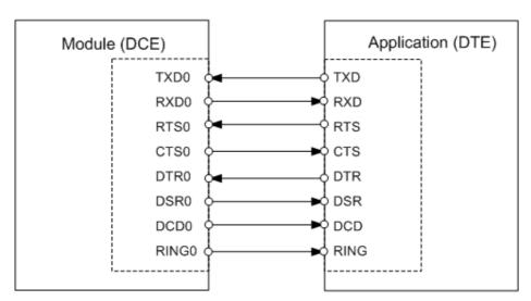
Figure 2: Serial interface ASC0
