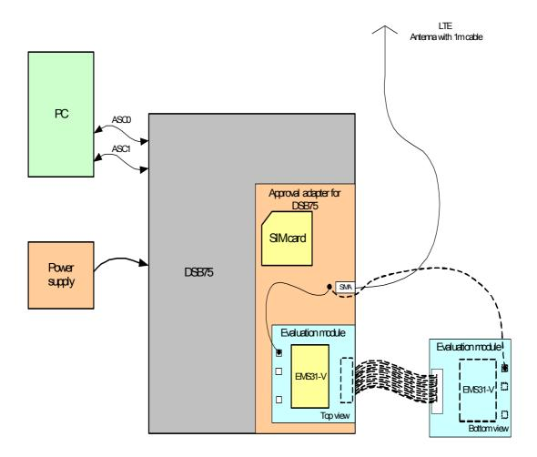
Figure 9: Reference equipment for Type Approval
