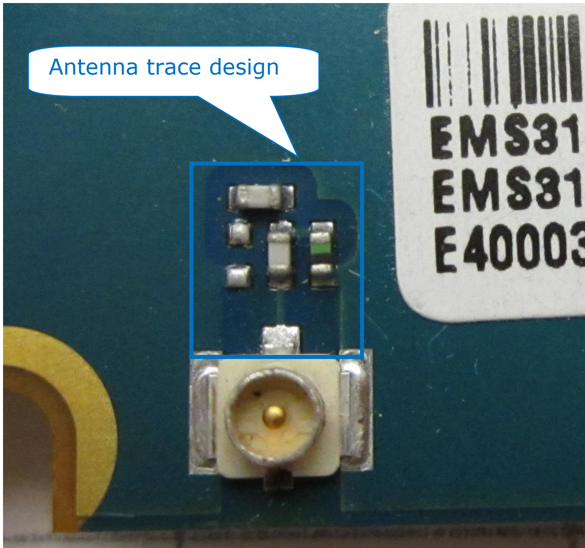
Photo 5: Module Antenna trace design
