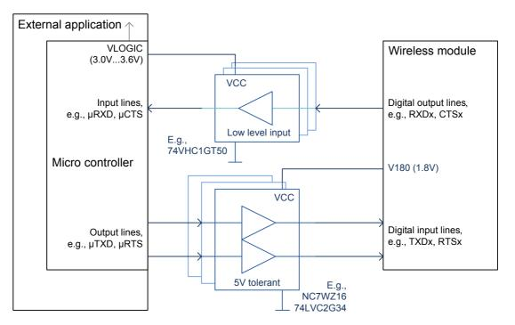
Figure 28: Sample level conversion circuit
