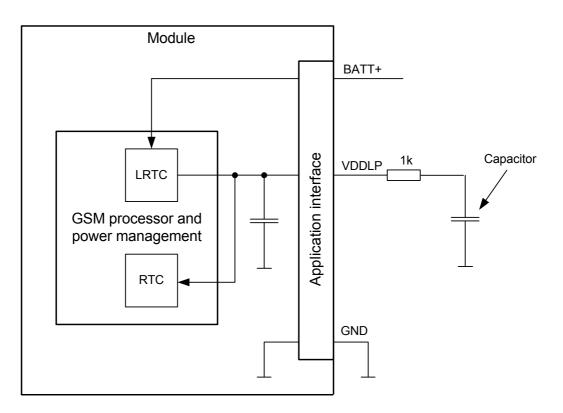
Figure 12: RTC supply variants
