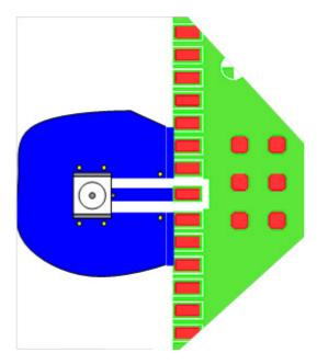
Figure 26: Routing to application's RF connector - top view
