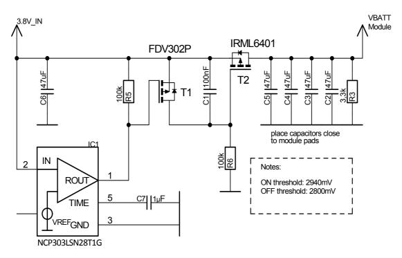
Figure 30: Sample circuit for applying power using an external voltage supervisory circuit
