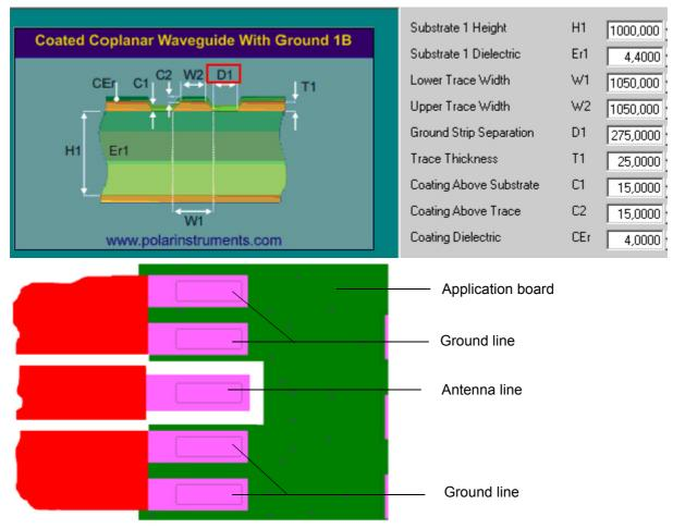
Figure 23: Micro-Stripline on 1.0mm Standard FR4 PCB - example 2
