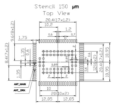
Figure 45: Recommended design for 150µm micron thick stencil (top view)
