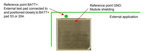
Figure 38: Position of reference points BATT+ and GND
