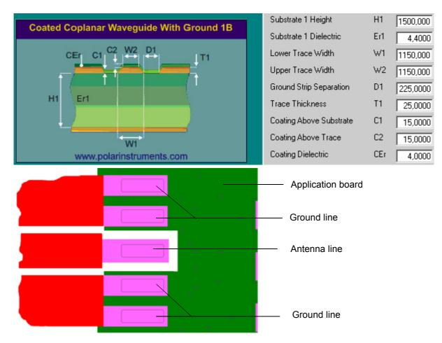
Figure 25: Micro-Stripline on 1.5mm Standard FR4 PCB - example 2
