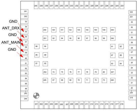
Figure 20: Antenna pads (bottom view)
