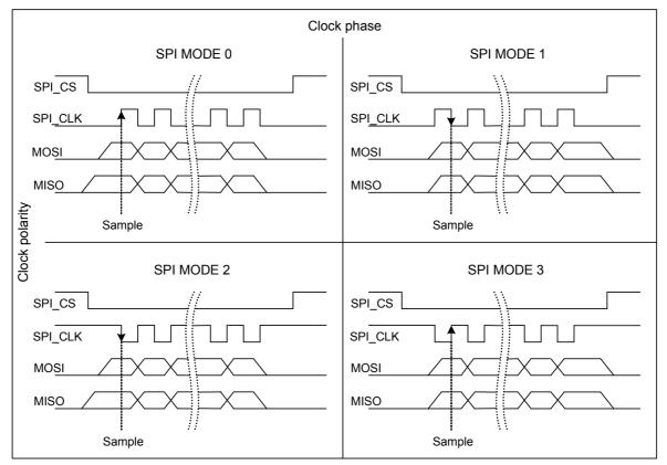
Figure 16: Characteristics of SPI modes
