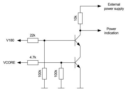
Figure 18: Power indication circuit
