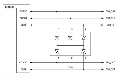
Figure 11: SIM interface - enhanced ESD protection
