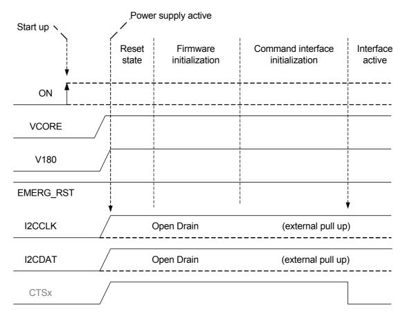
**Figure 15:** I<sup>2</sup>C startup behavior
