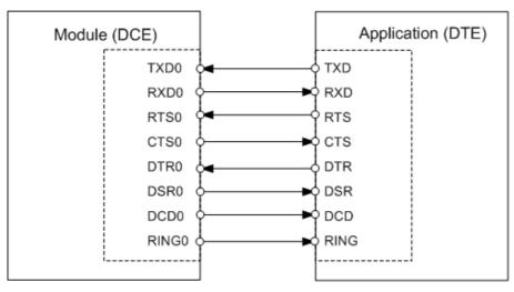
Figure 6: Serial interface ASC0
