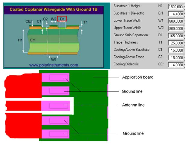
Figure 24: Micro-Stripline on 1.5mm Standard FR4 PCB - example 1
