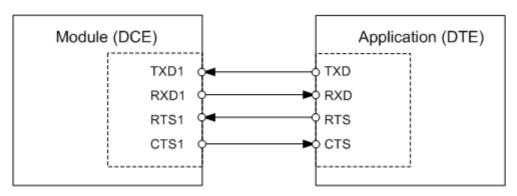
Figure 8: Serial interface ASC1
