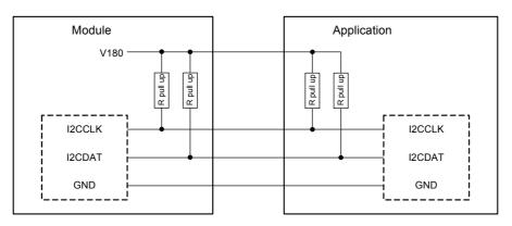
**Figure 14:** I<sup>2</sup>C interface connected to V180
