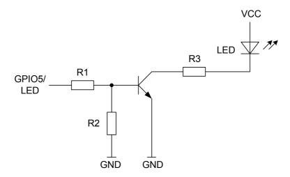
Figure 17: Status signaling with LED driver
