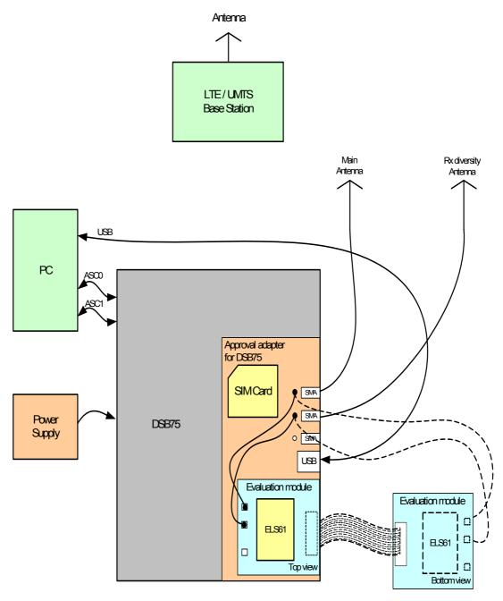
Figure 54: Reference equipment for Type Approval
