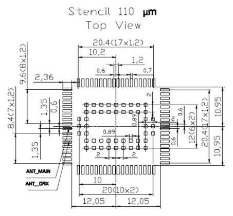
Figure 44: Recommended design for 110µm micron thick stencil (top view)
