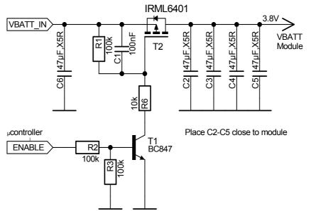
Figure 29: Sample circuit for applying power using an external µC
