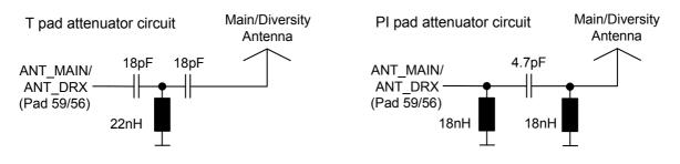
Figure 39: ESD protection for RF antenna interface
