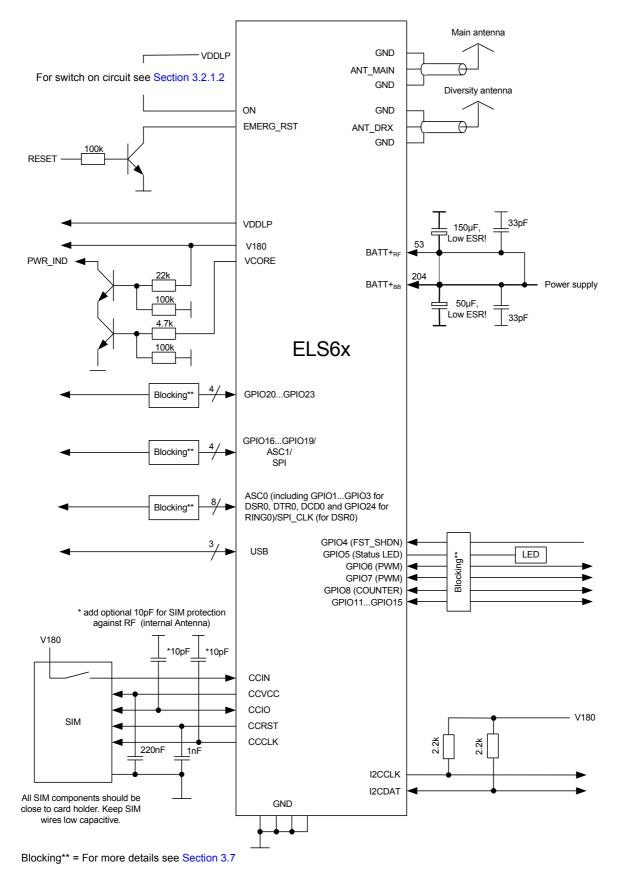
Figure 27: Schematic diagram of ELS61-AUS sample application
