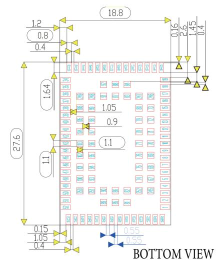
Figure 15: Dimensions of ELS31-US/ELS51-US (all dimensions in mm) - bottom view
