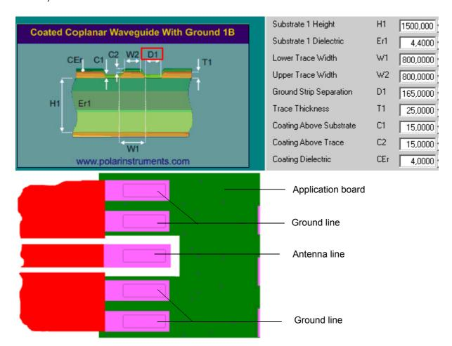
Figure 10: Micro-Stripline on 1.5mm Standard FR4 PCB - example 1
