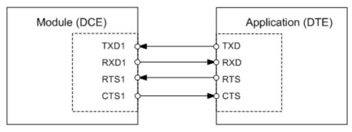
Figure 4: Serial interface ASC1
