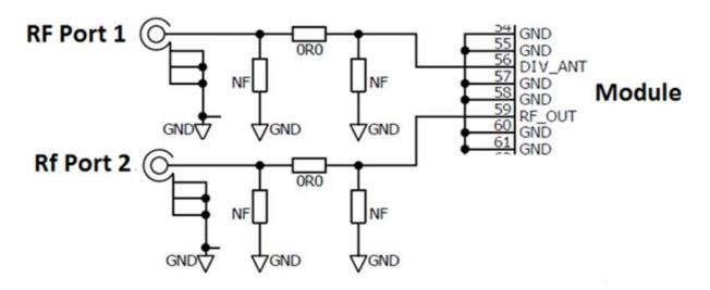
Figure 6: RF interface signals example
