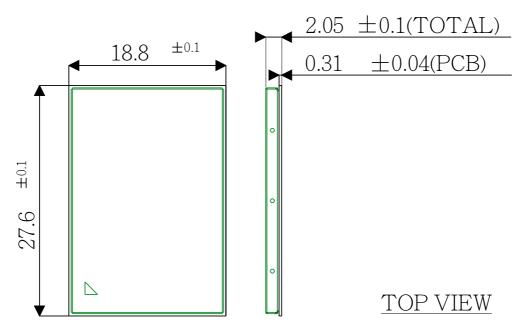
Figure 14: Dimensions of ELS31-US/ELS51-US (all dimensions in mm)
