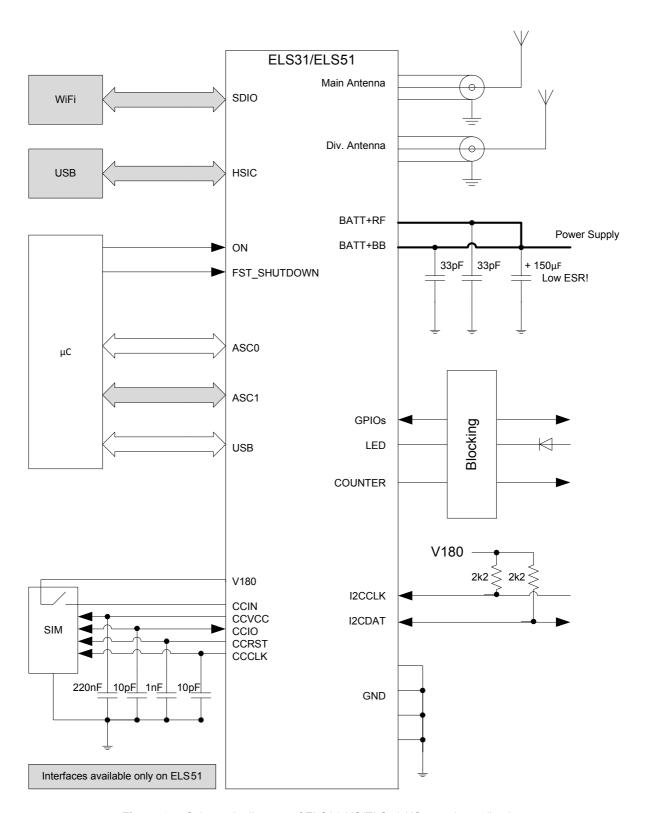
Figure 12: Schematic diagram of ELS31-US/ELS51-US sample application
