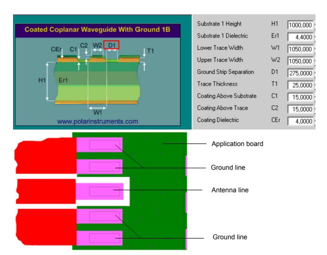
Figure 9: Micro-Stripline on 1.0mm Standard FR4 PCB - example 2
