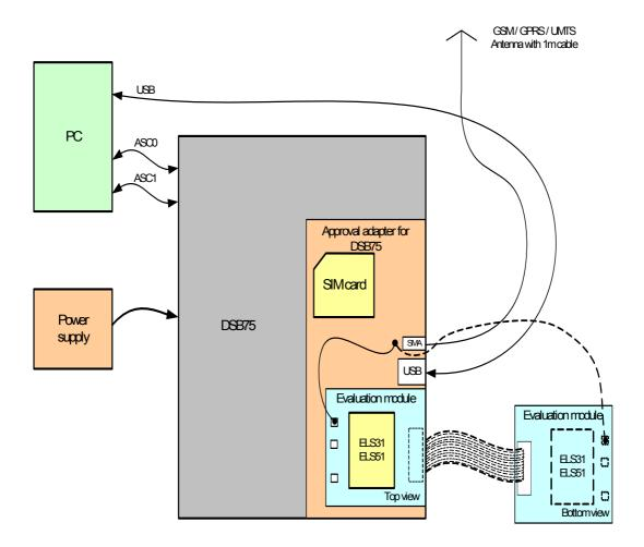
Figure 16: Reference equipment for Type Approval
