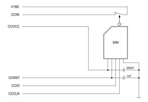
Figure 5: External UICC/SIM/USIM card holder circuit
