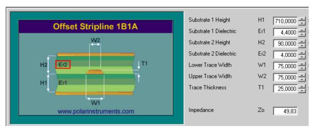
Figure 7: Embedded Stripline with 65μm prepreg (1080) and 710μm core
