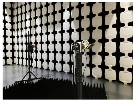
Description: Substitution Antenna for EIRP Test
