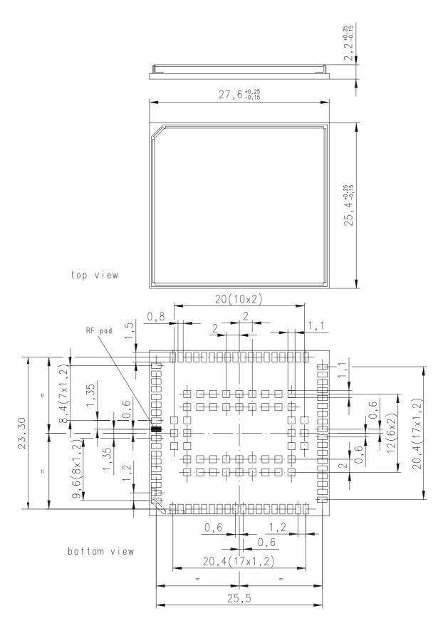
Figure 8: Dimensions of EHS8 (all dimensions in mm)
