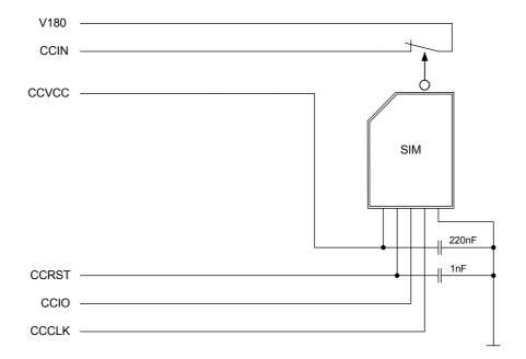
Figure 5: External UICC/SIM/USIM card holder circuit
