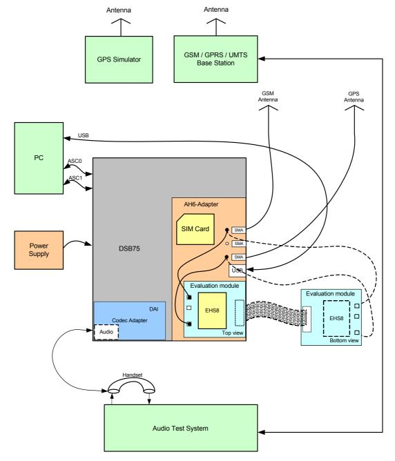
Figure 9: Reference equipment for Type Approval
