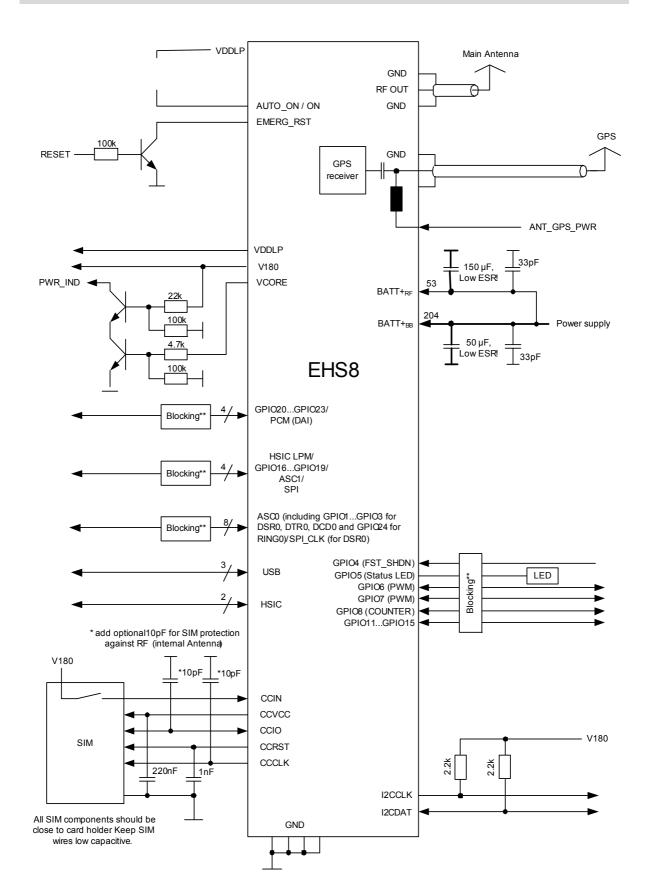
Figure 6: Schematic diagram of EHS8 sample application
