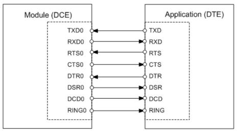
Figure 3: Serial interface ASC0
