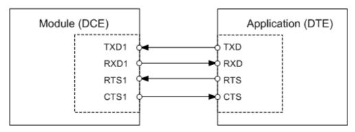
Figure 4: Serial interface ASC1
