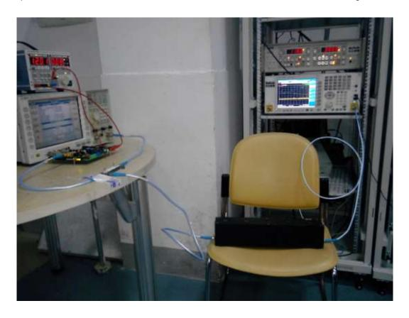
Frequency Stability Under Temperature & Voltage Variations Setup
