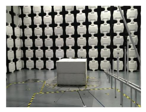
Test Mode: Mode 1 Description: Backview of Radiated Emission Test Setup
