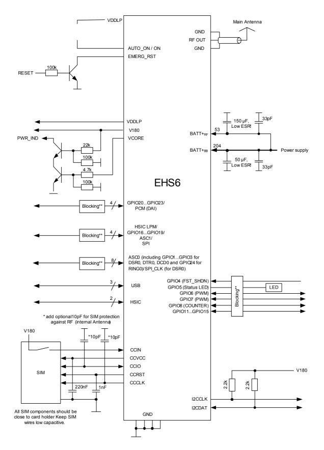
Figure 6: Schematic diagram of EHS6 sample application
