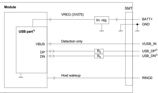
All serial (including R<sub>s</sub>) and pull-up resistors for data lines are implemented.
