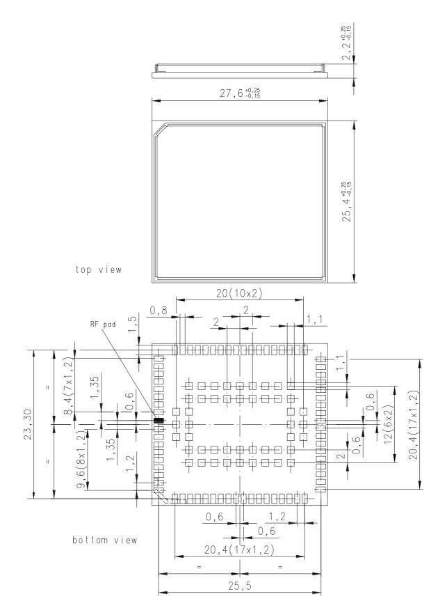
Figure 8: Dimensions of EHS6 (all dimensions in mm)
