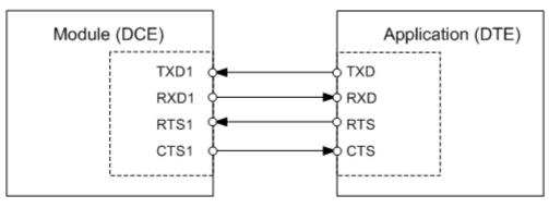
Figure 4: Serial interface ASC1
