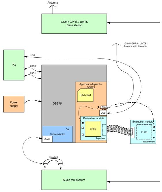
Figure 9: Reference equipment for Type Approval
