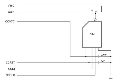
The figure below shows a circuit to connect an external SIM card holder.
