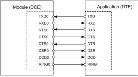
Figure 3: Serial interface ASC0
