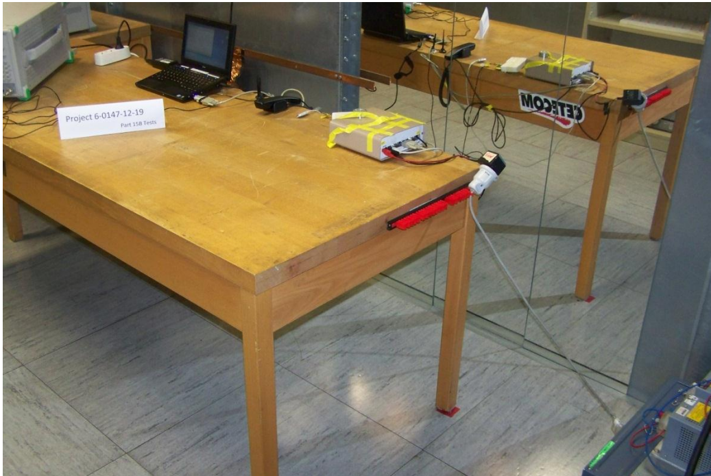
Conducted emissions measurements on AC-mains (test report 6-0147-19-6c)
