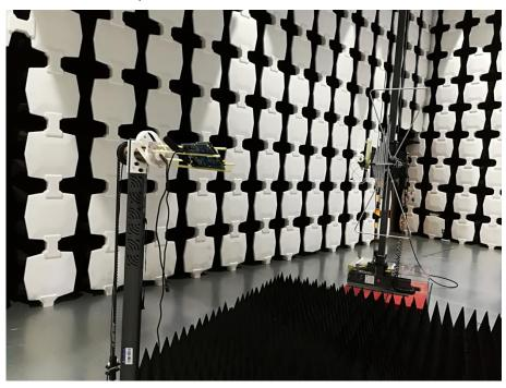
Description: Substitution Antenna for ERP Test
