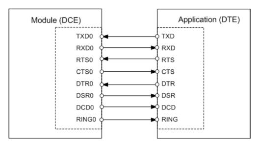
Figure 3: Serial interface ASC0
