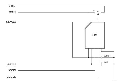
Figure 5: External UICC/SIM/USIM card holder circuit
