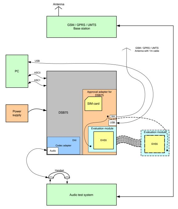
Figure 9: Reference equipment for Type Approval
