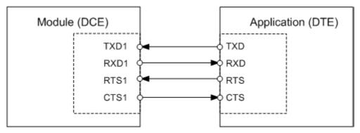
Figure 4: Serial interface ASC1
