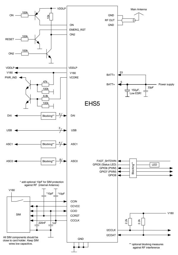
Figure 6: Schematic diagram of EHS5-E/EHS5-US sample application
