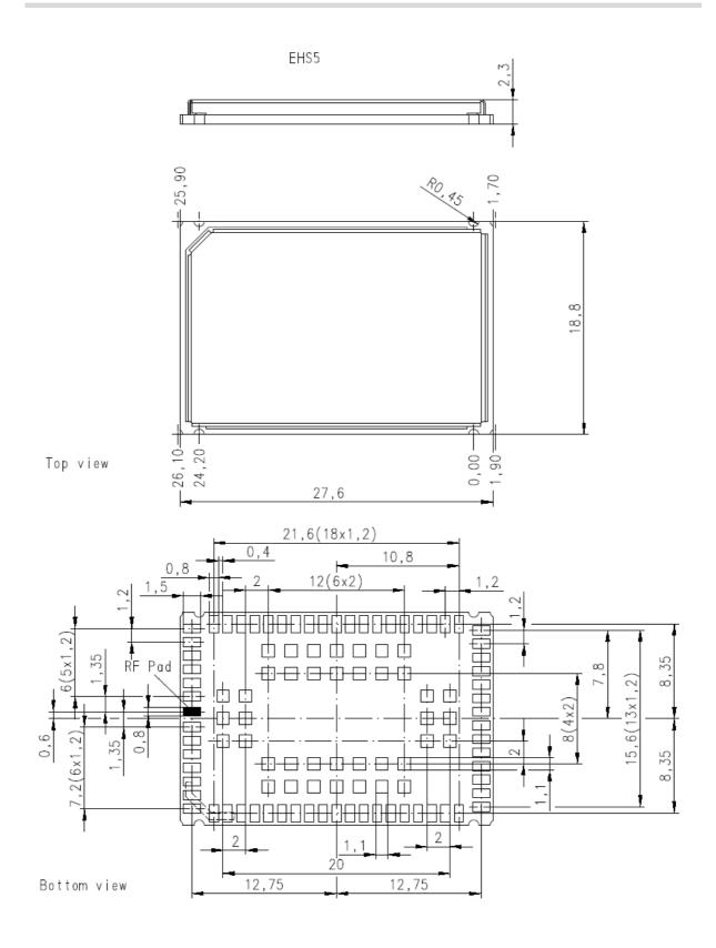
Figure 8: Dimensions of EHS5-E/EHS5-US (all dimensions in mm)
