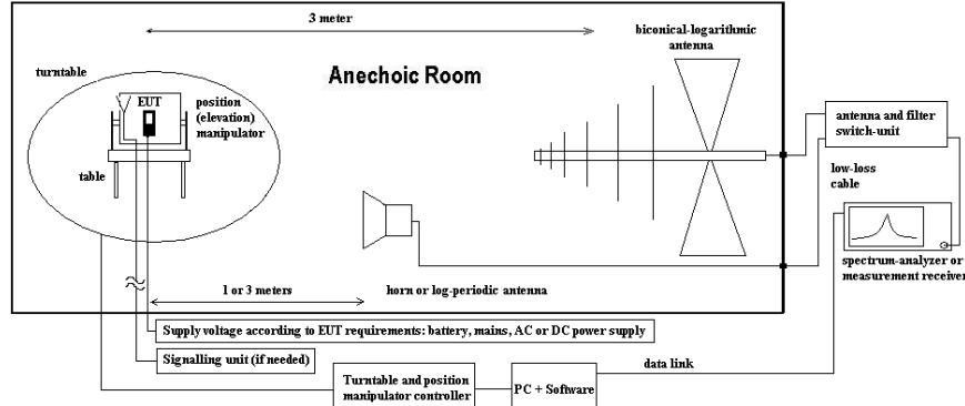
**Testing method:****Exploratory, preliminary measurements**
