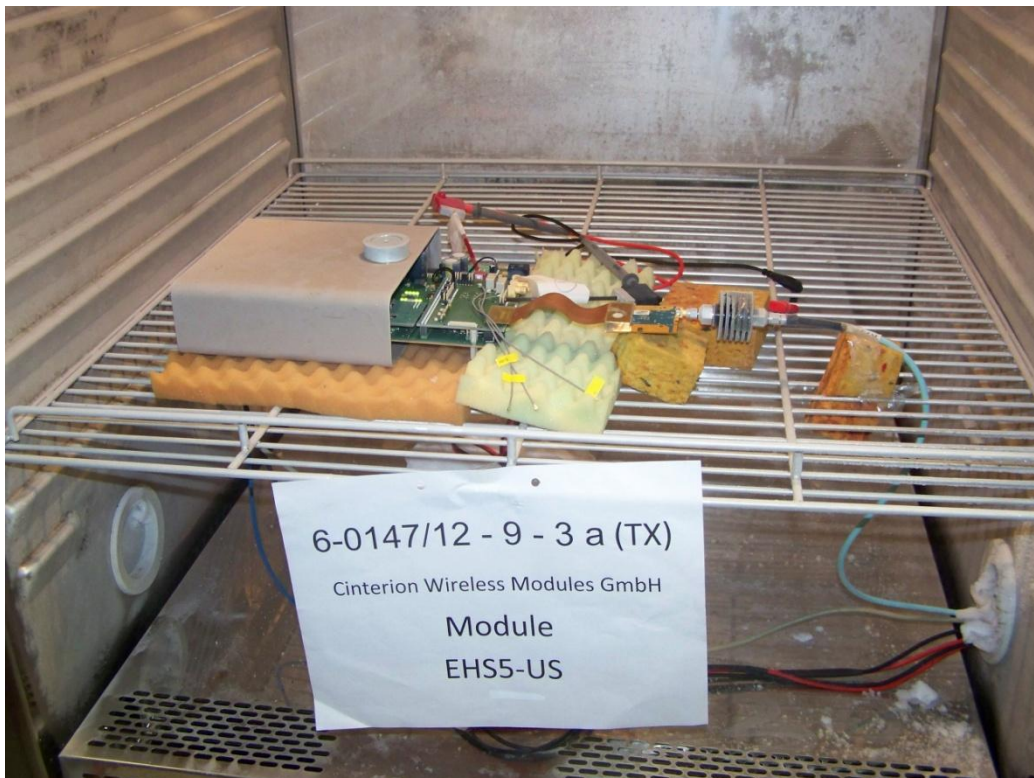
Conducted emissions measurements in the Radio laboratory 1 (incl. climatic tests), test setup 2.
