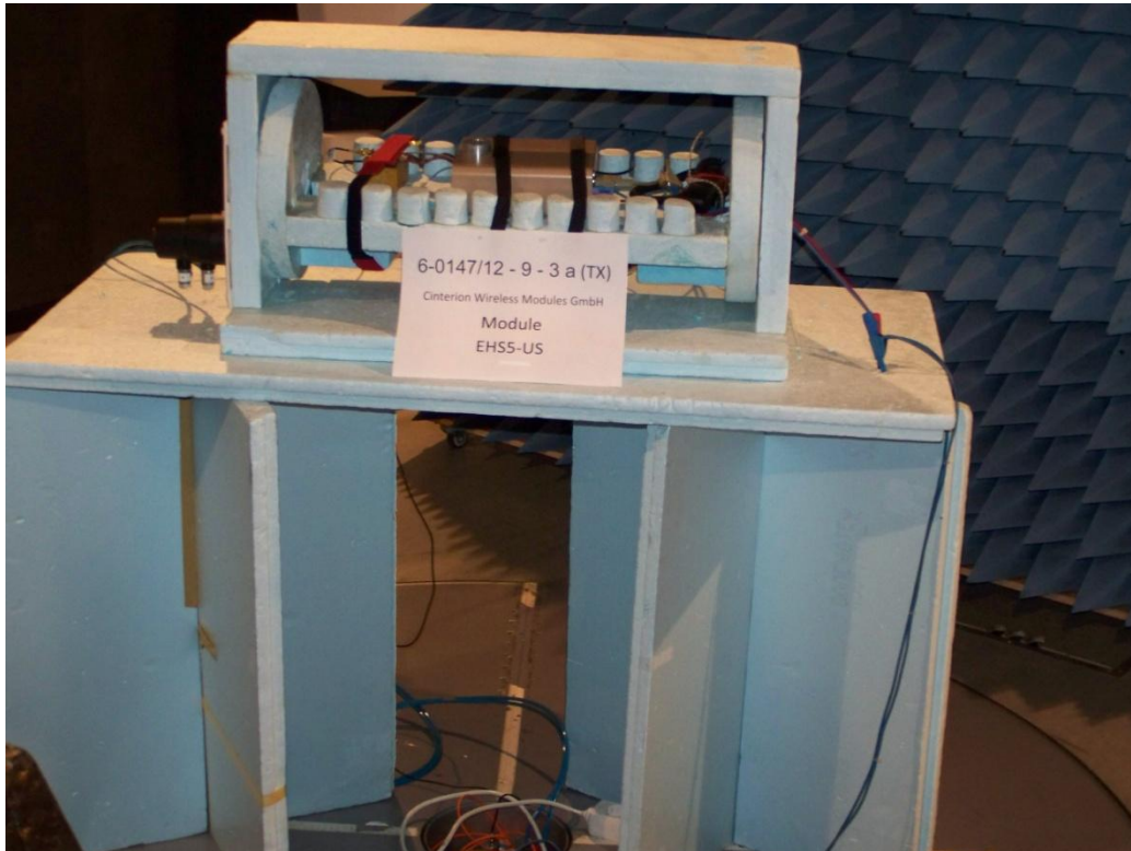
Radiated field strength measurements in the SAR (Semi-Anechoic-Chamber), test setup 2
