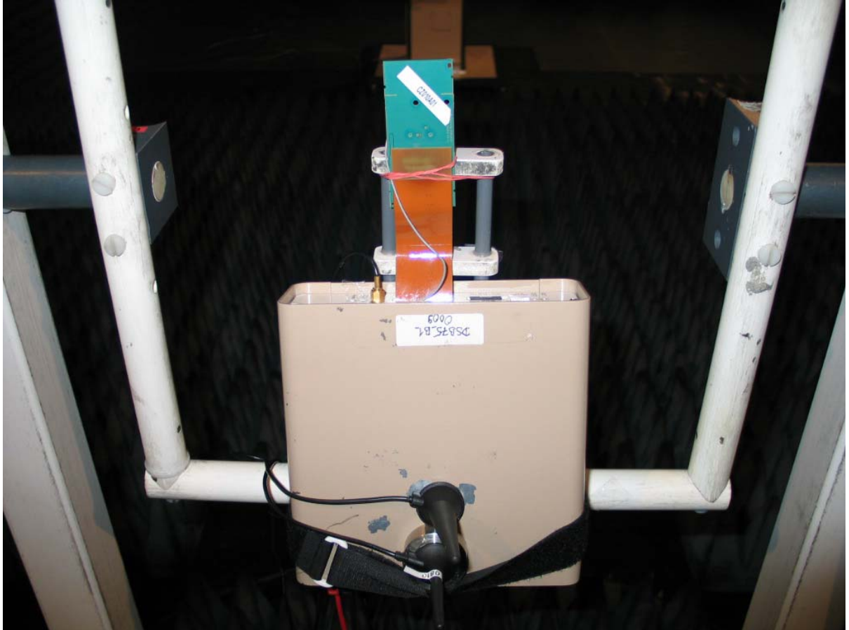
setup for radiated tests
