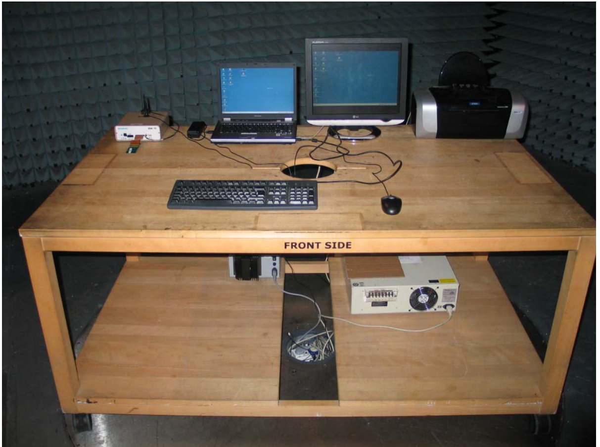
set-up for radiated tests
