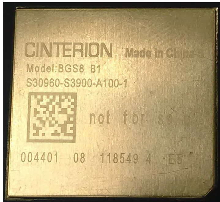
BGS8 - label location lasing on shielding
