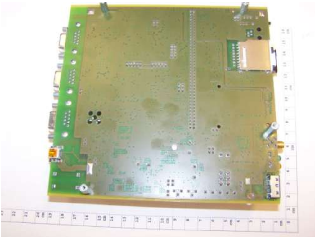
Photograph 10: DSB 75 V1.1 board - bottom site (EUT E)
