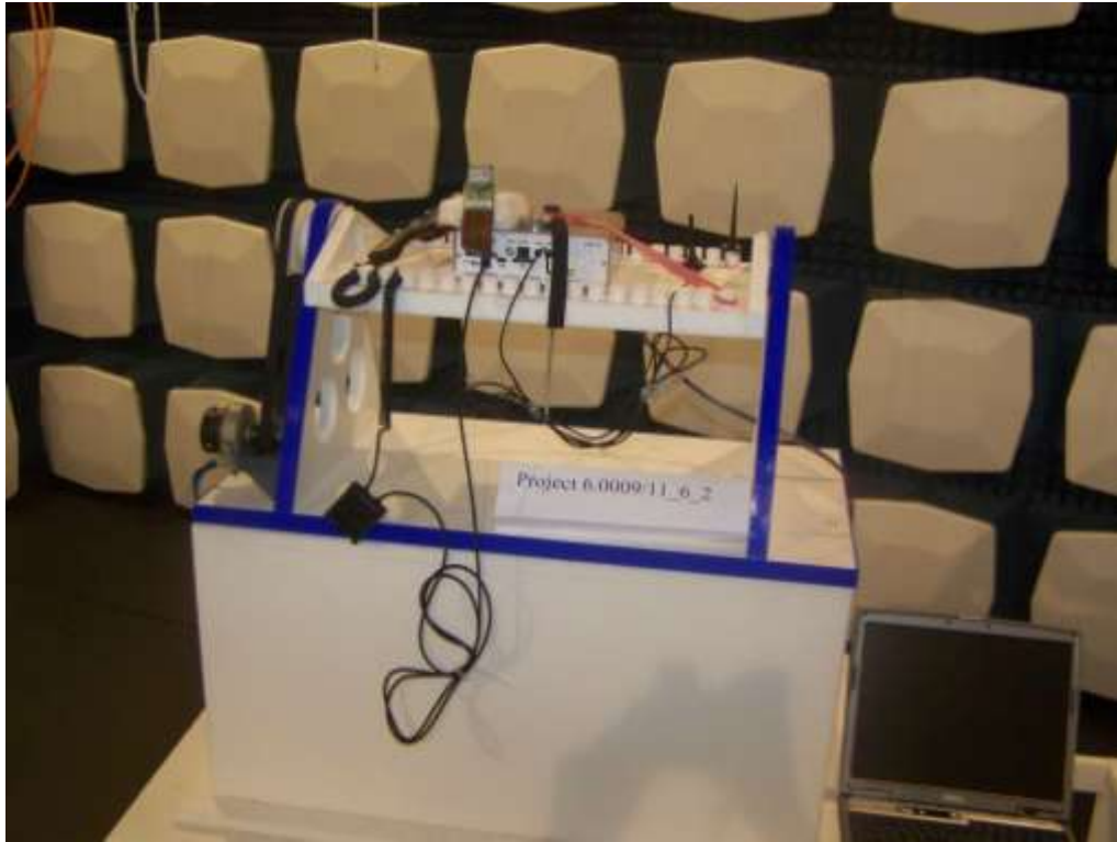
Photograph 2: Radiated measurement set-up at FAR (Fully-Anechoic-Room)
