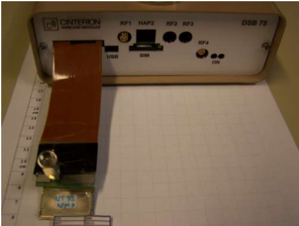
Photograph: Modules connection (control and power lines) to DSB75 Box
