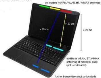
**Important note**: this notebook configuration is an example. Different applications (e.g. M2M) are also possible as long as the same antenna-to-antenna and antenna-to-user distances are respected.
