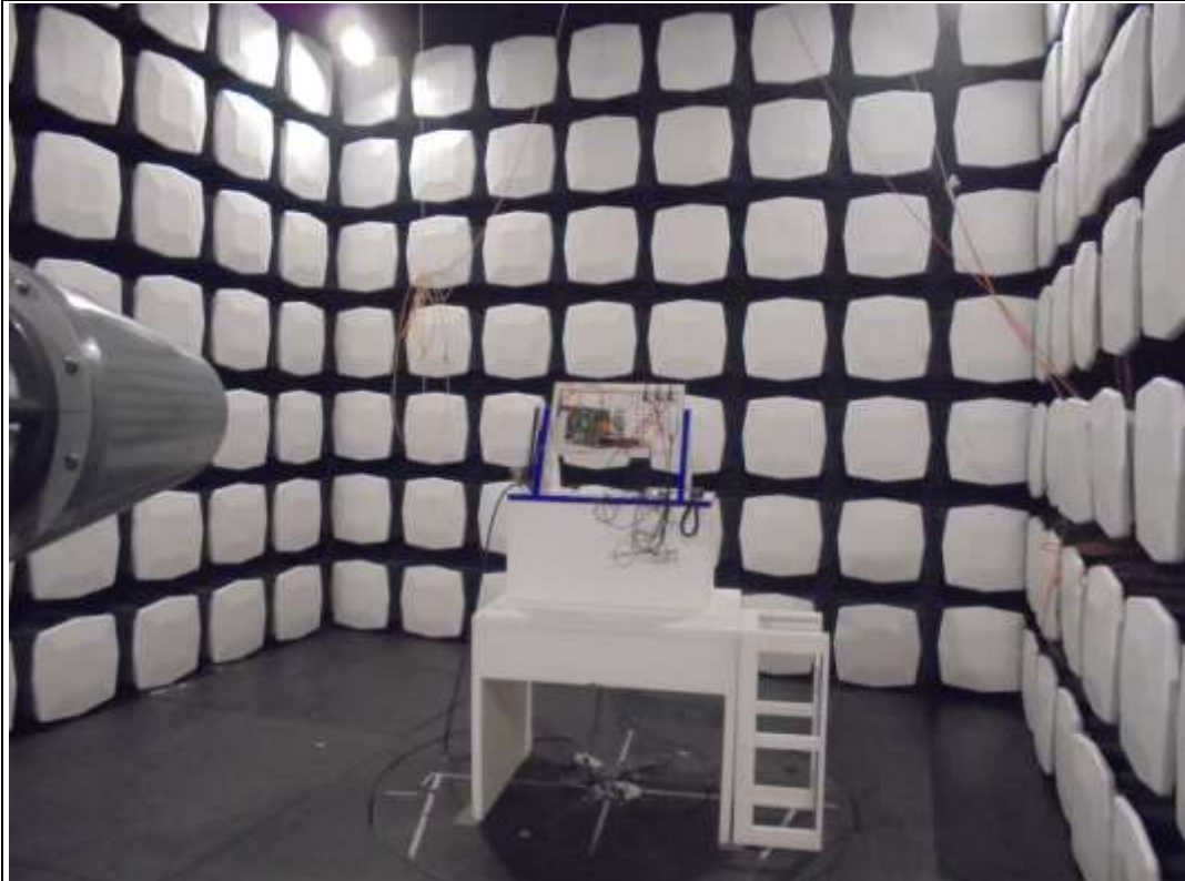
Photograph 5: Test set-up for radiated measurements (overview)
