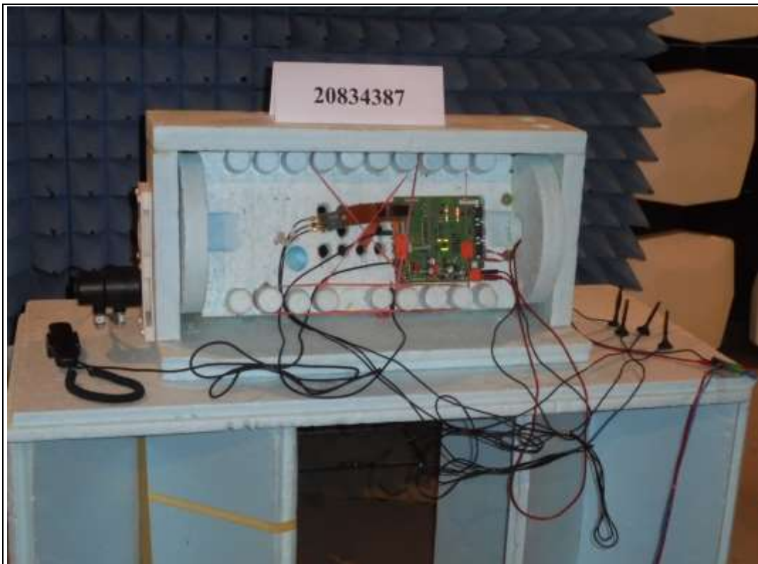
Photograph 2: Radiated measurements test set-up, magnetic field strengths
