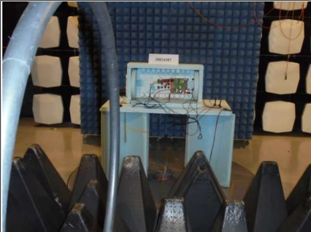
Photograph 3: Radiated measurements test set-up, magnetic field strengths (overview)
